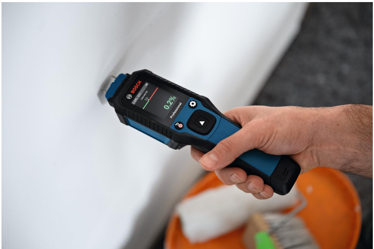
Figure 4: Detailed view of the device pins inserted into a wall surface during measurement.
