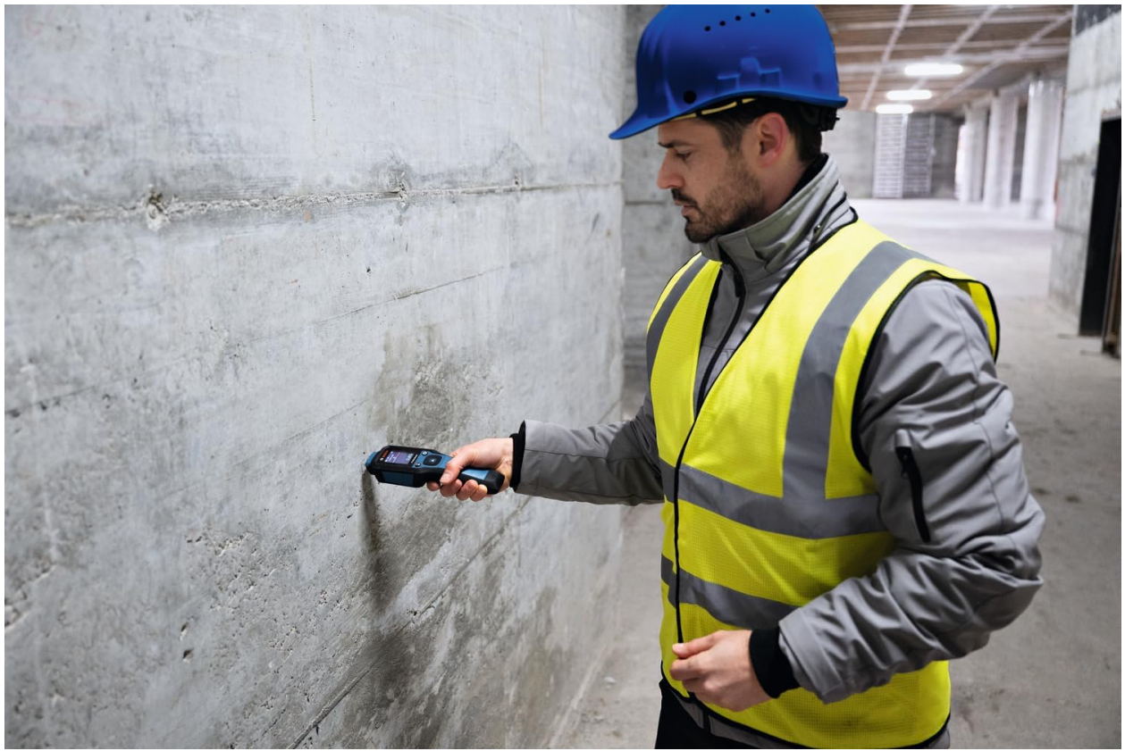
Figure 3: Measuring moisture content in a concrete wall.
