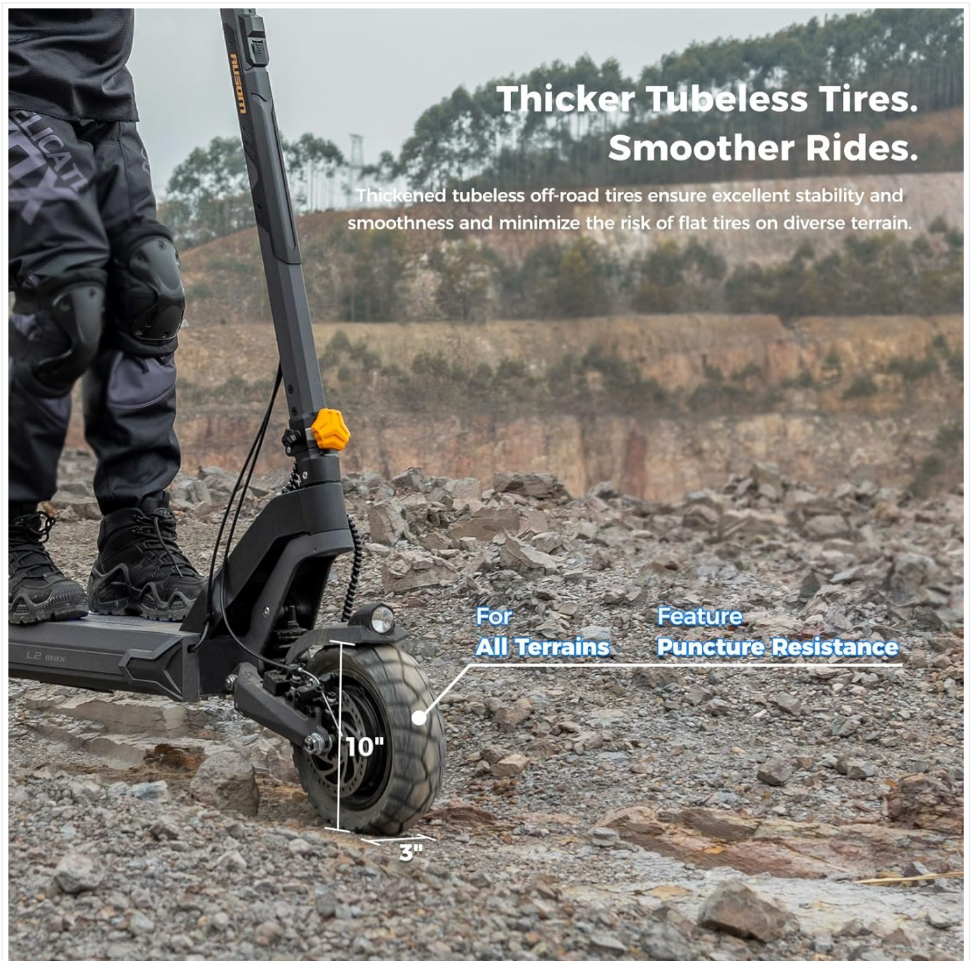
Figure 6.1: Tubeless Knobby Tires. These 10-inch tires are designed for off-road stability and puncture resistance, requiring regular inspection for optimal performance.
