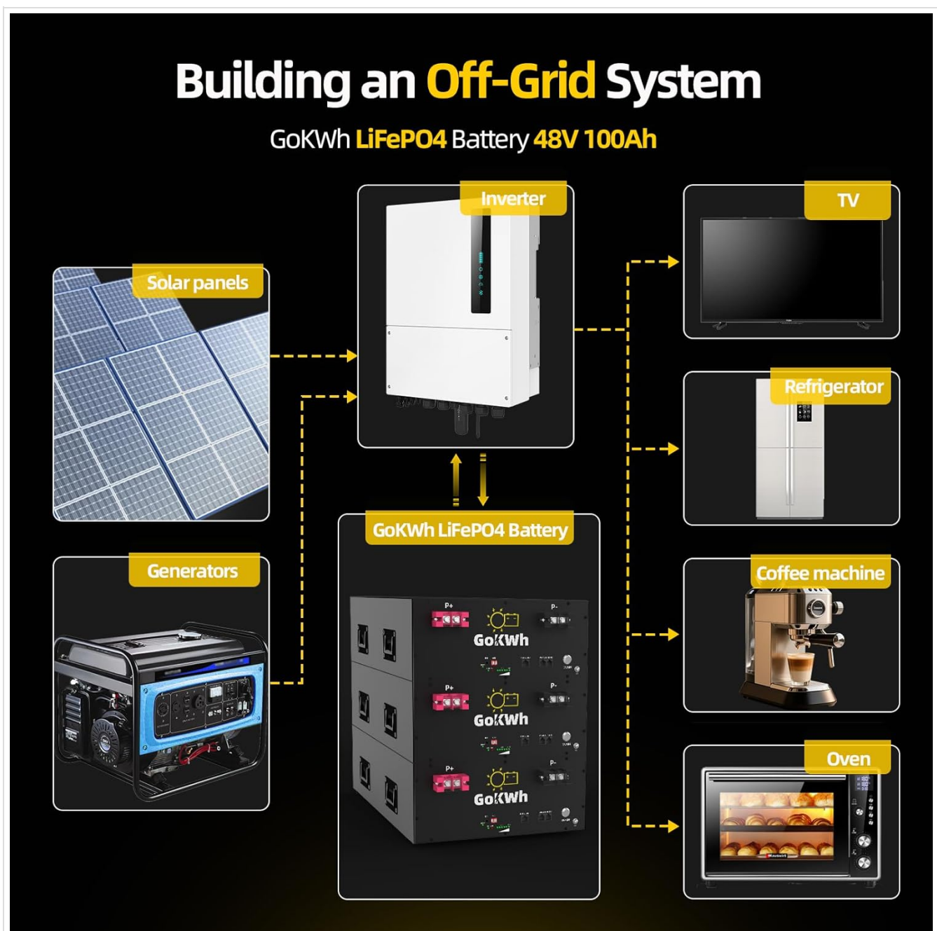
Image: A comprehensive diagram showing how the GOKWH LiFePO4 battery integrates into an off-grid system, connecting solar panels, generators, an inverter, and powering household appliances like TVs, refrigerators, coffee machines, and ovens.
