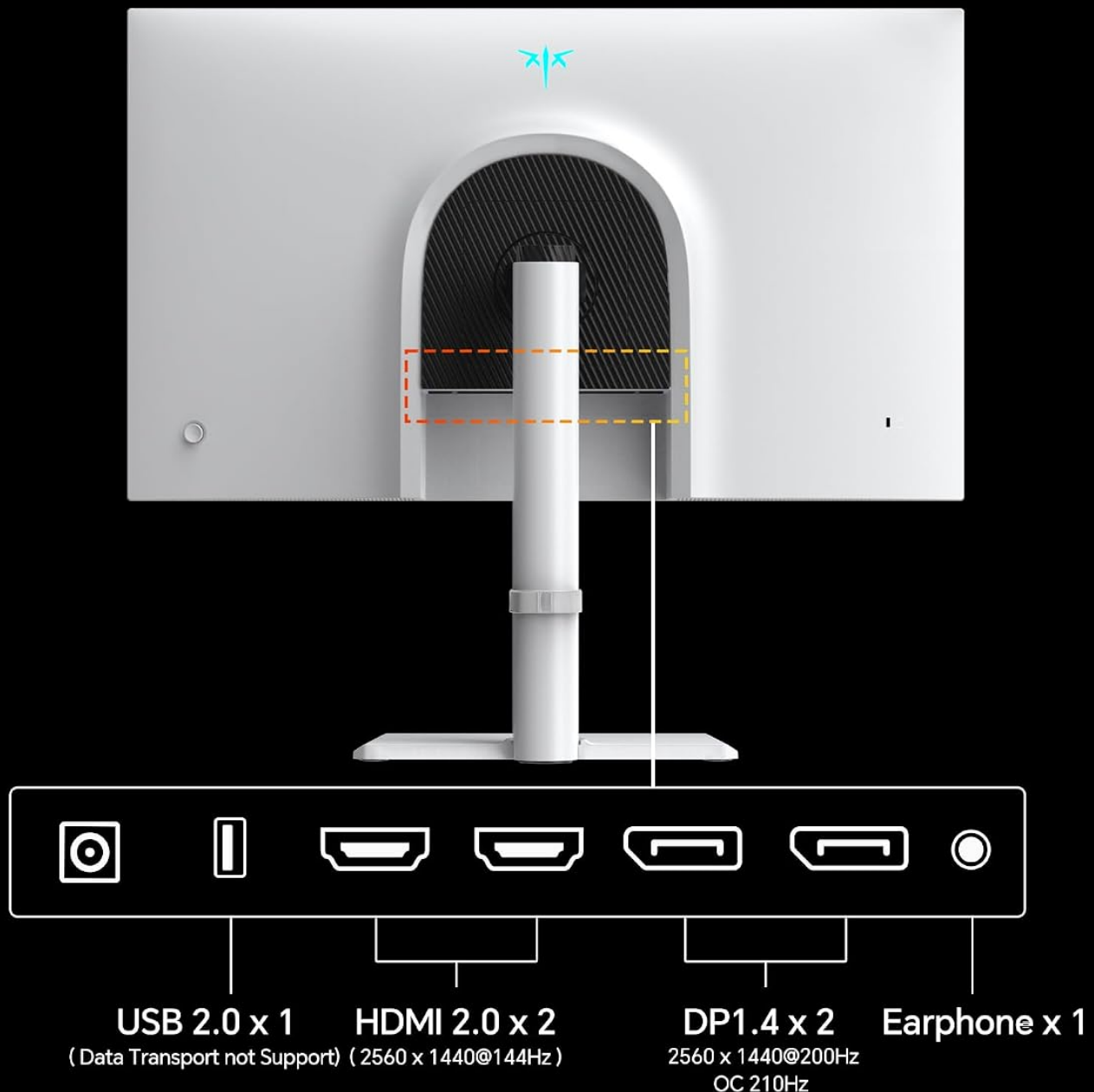
Image 3.2: Overview of the monitor's input and output ports.
