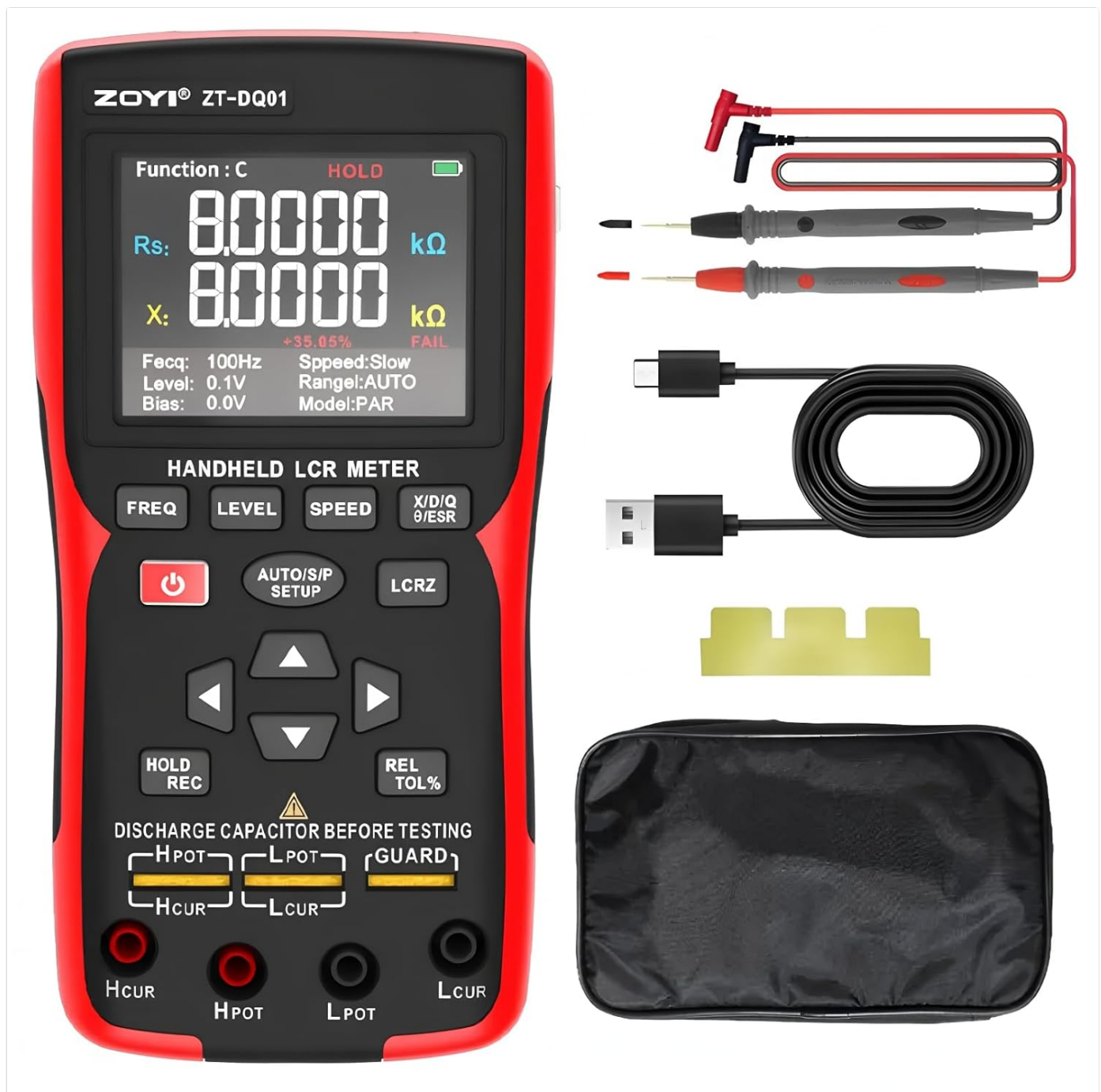
Image 1: FeelTech ZT-DQ01 LCR Meter and included accessories.
