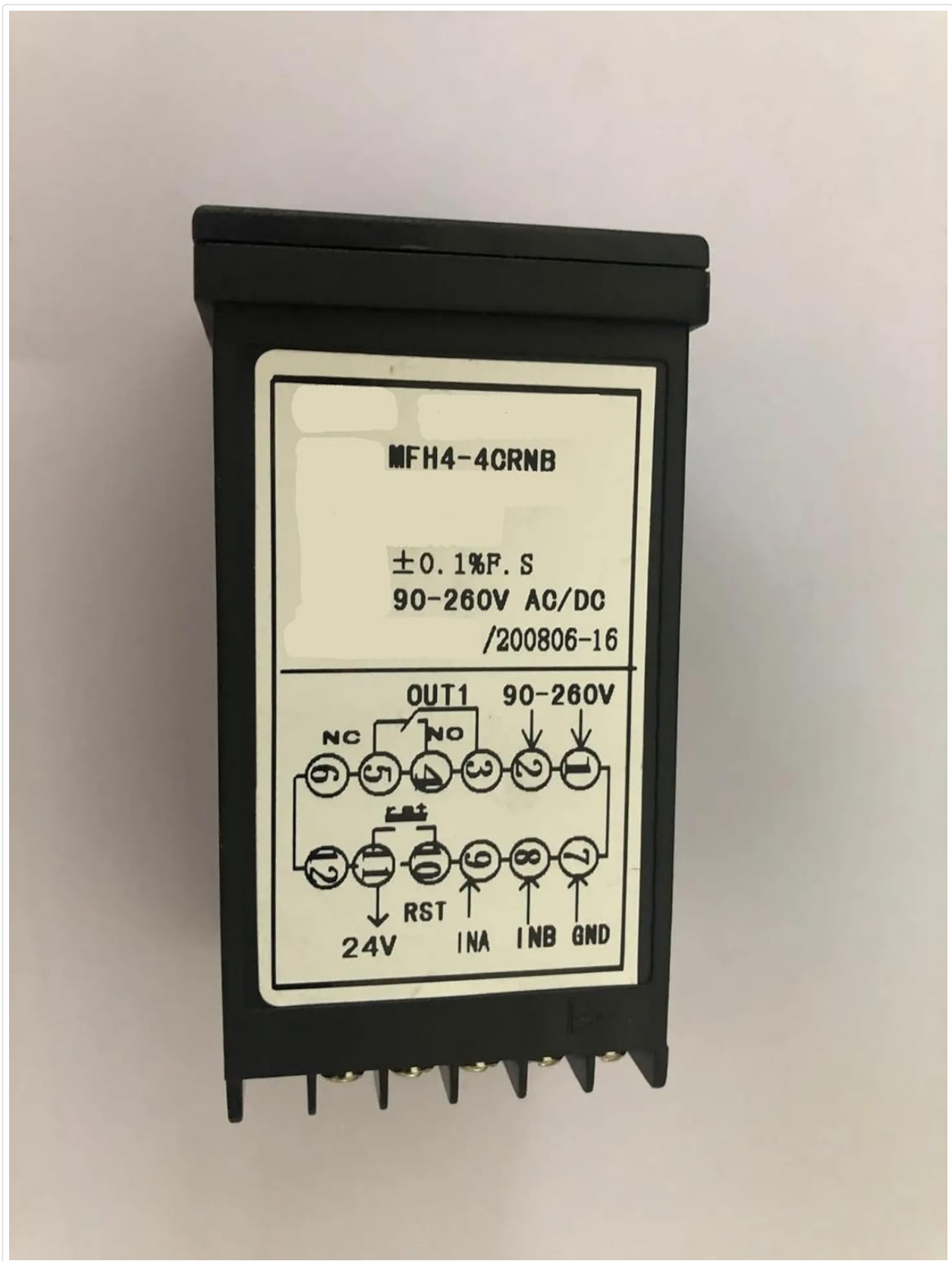
Figure 6.1: Side view of the FH4-4CRNB Digital Counter Meter showing the wiring diagram. This diagram details connections for power (90-260V AC/DC), relay output (OUT1: NC, NO, COM), reset (RST), 24V auxiliary power, and signal inputs (INA, INB, GND).
