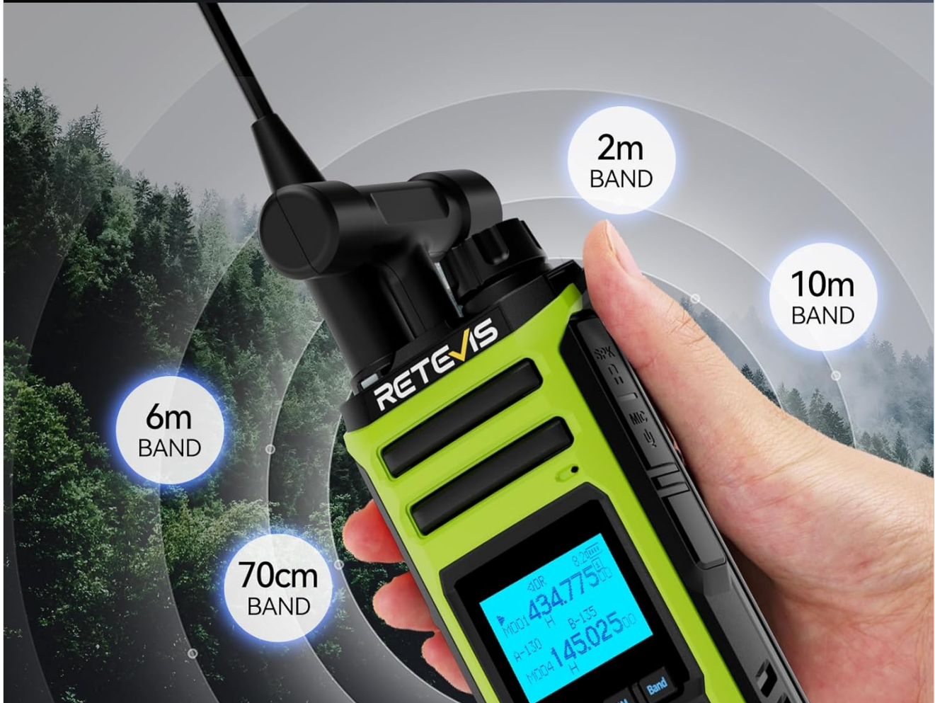
Figure 2.2: The Retevis A3 supports quad-band transmission across 10m, 6m, 2m, and 70cm bands.
