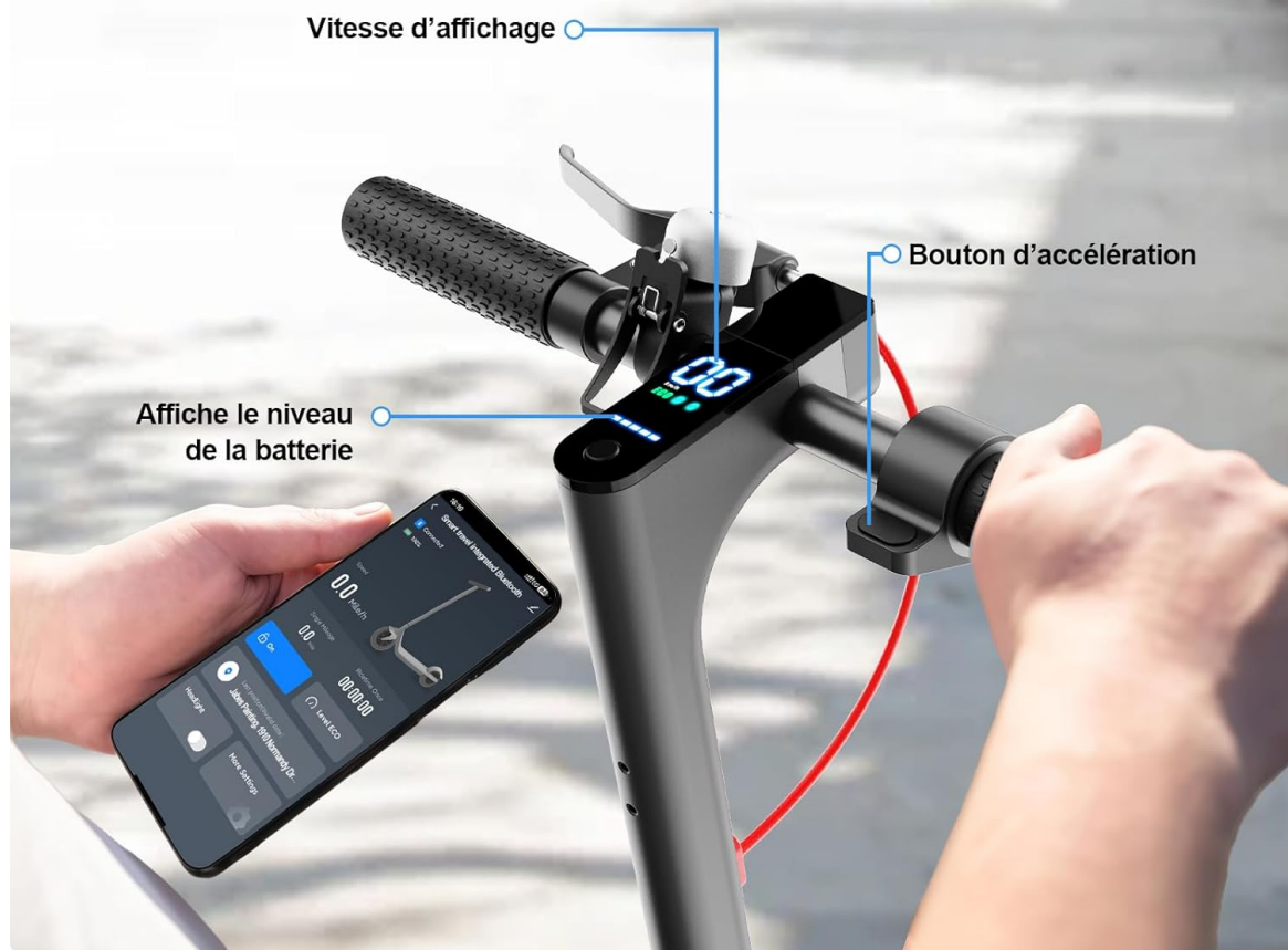
Figure 4.3: Detail of the handlebars, showing the integrated LCD display for speed and battery level, and the acceleration button for control.
