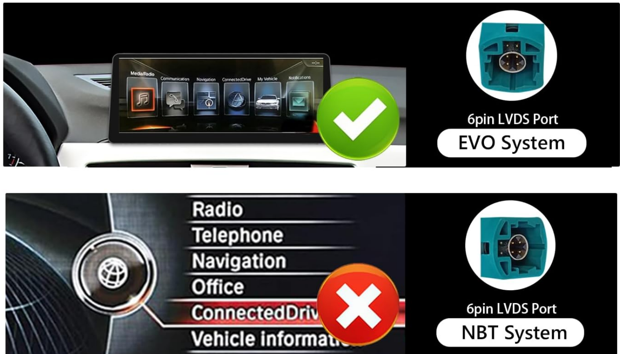
Figure 3.1: Visual guide for identifying compatible BMW X1 F48 EVO System (6pin LVDS Port) versus incompatible NBT System.
