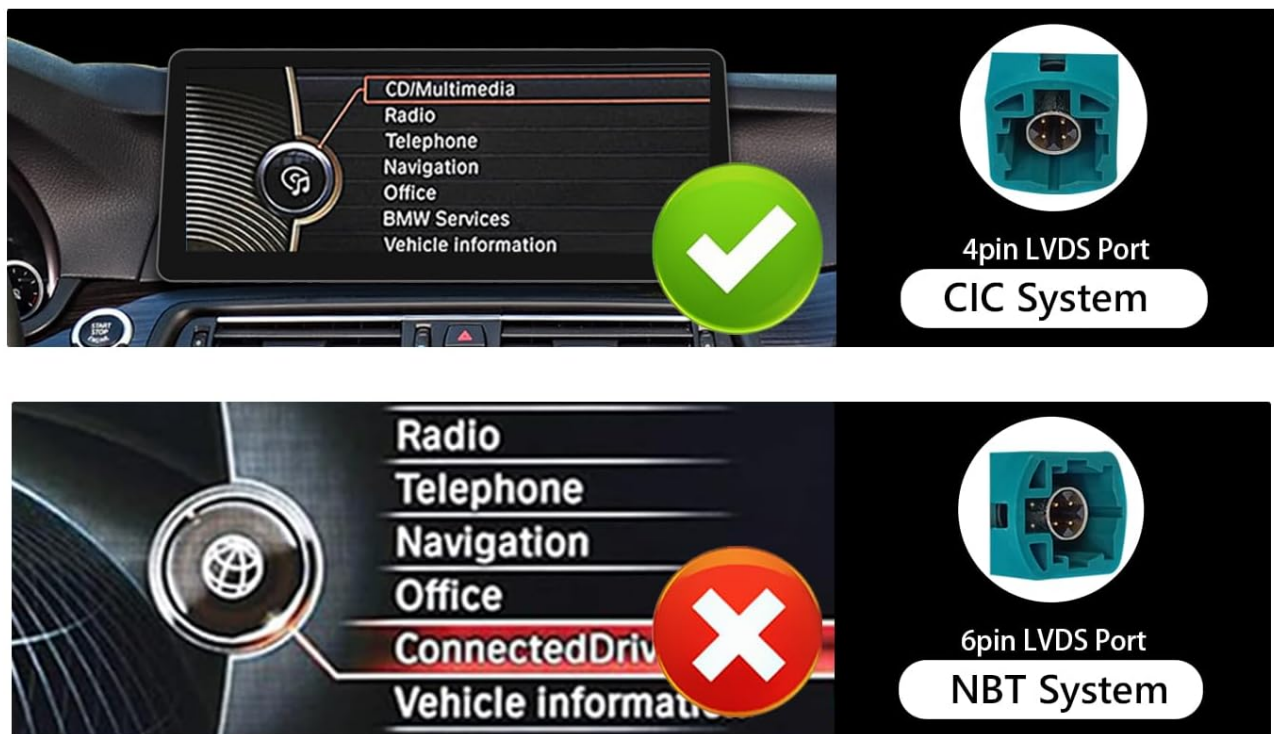
Figure 8: Guide to identify your BMW system: CIC systems typically have a 4-pin LVDS port, while NBT systems have a 6-pin LVDS port. Ensure your vehicle has the correct CIC system for compatibility.
