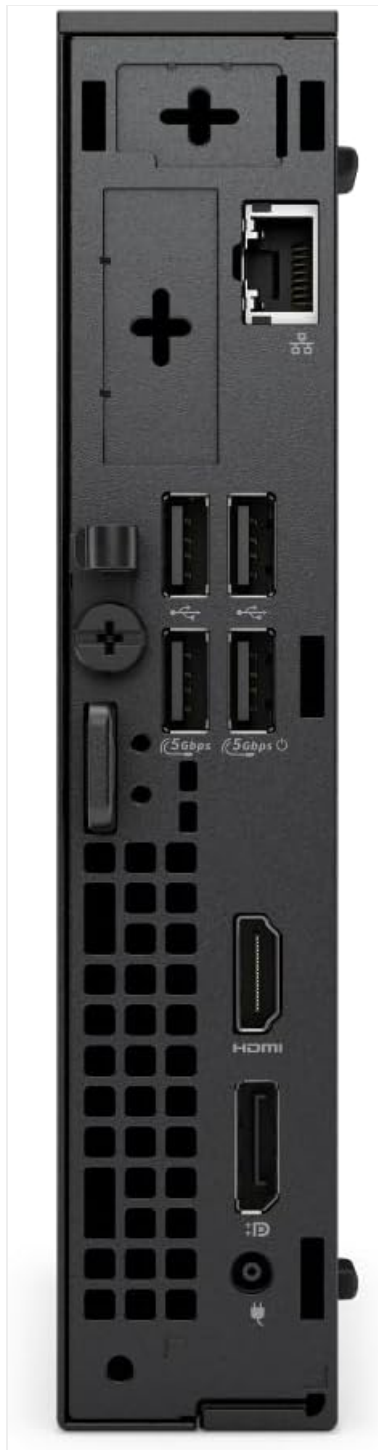
Image: Rear Ports. This image shows the rear panel of the Dell Pro Micro QCM1250 Mini PC, detailing the Ethernet (RJ-45) port, two USB 2.0 Type-A ports, two USB 3.2 Type-A ports (5Gbps), HDMI 2.1 port, and DisplayPort.
