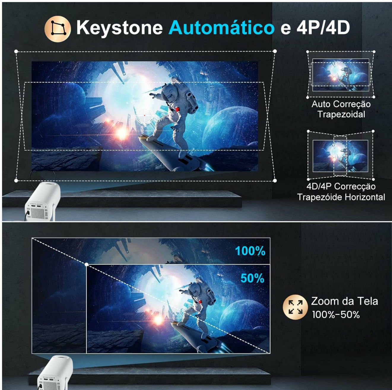
Figure 4.2: Illustration of keystone correction and digital zoom functionality on the JIFAR JP24 Projector, showing how to adjust image shape and size.
