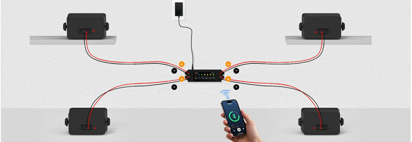
Image: Connection diagram illustrating how to wire four speakers to the amplifier and connect a mobile device via Bluetooth.
