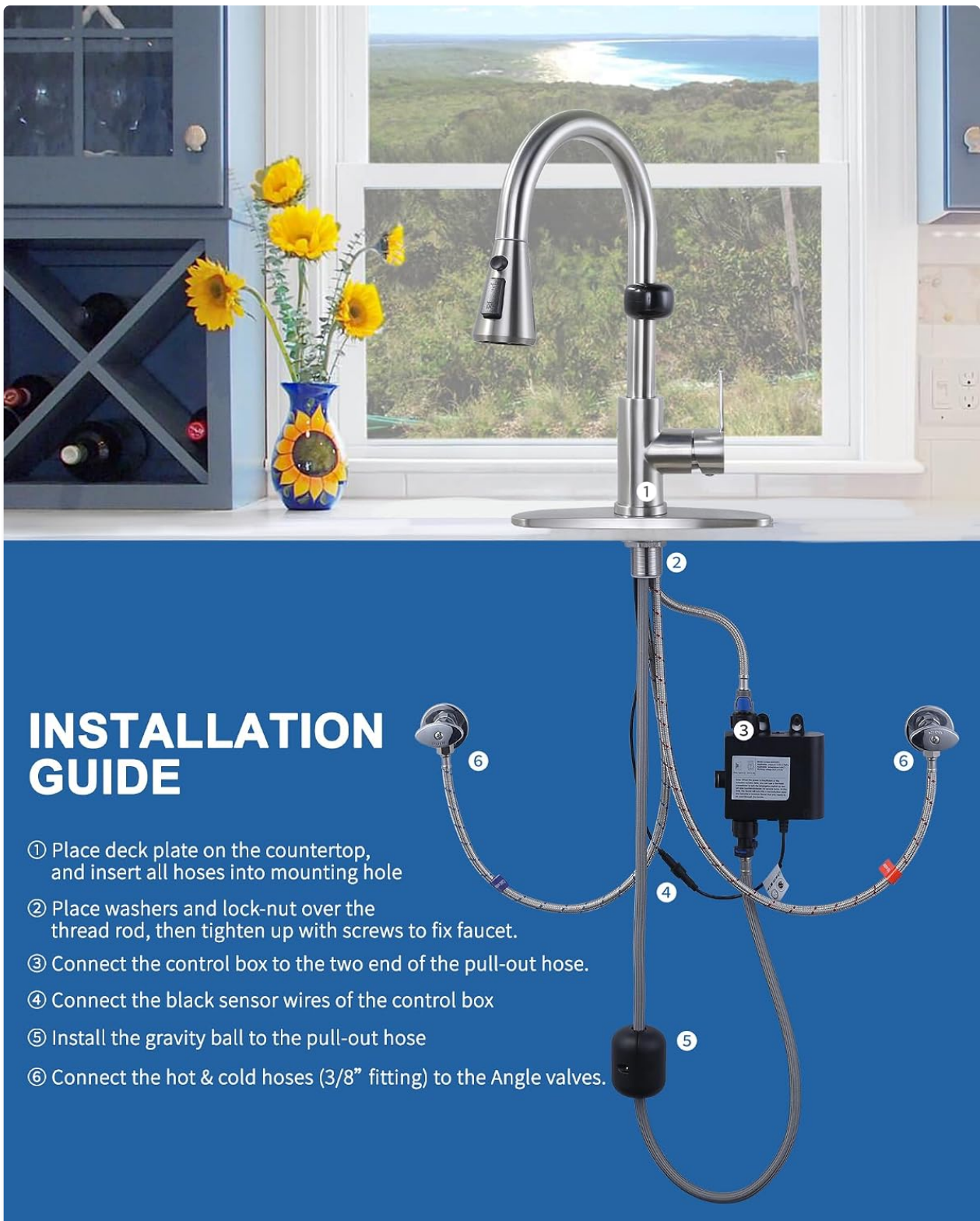
Image: Diagram illustrating the six steps for installing the ALEASHA touchless kitchen faucet, showing the connection points for hoses, control box, and gravity ball.
