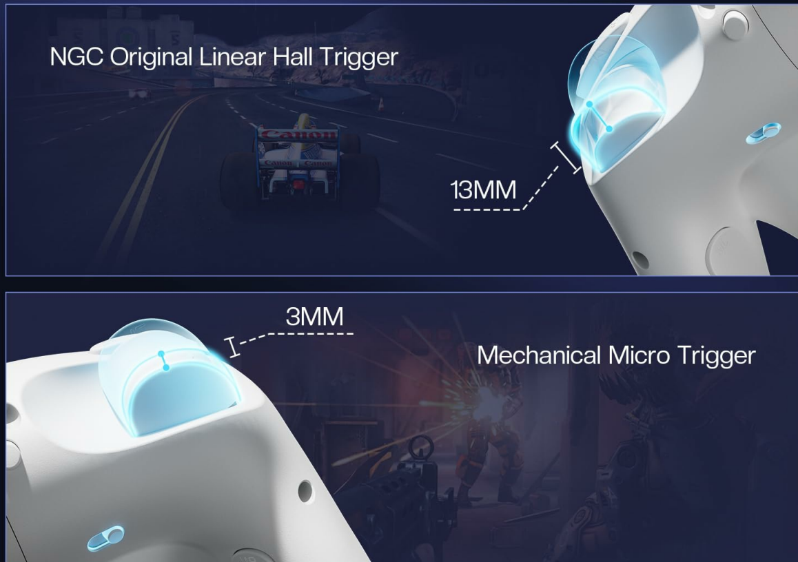
Image 4: This image visually compares the NGC Original Linear Hall Trigger, showing its 13mm travel for analog input, with the Mechanical Micro Trigger, which has a shorter 3mm actuation for faster digital response.
