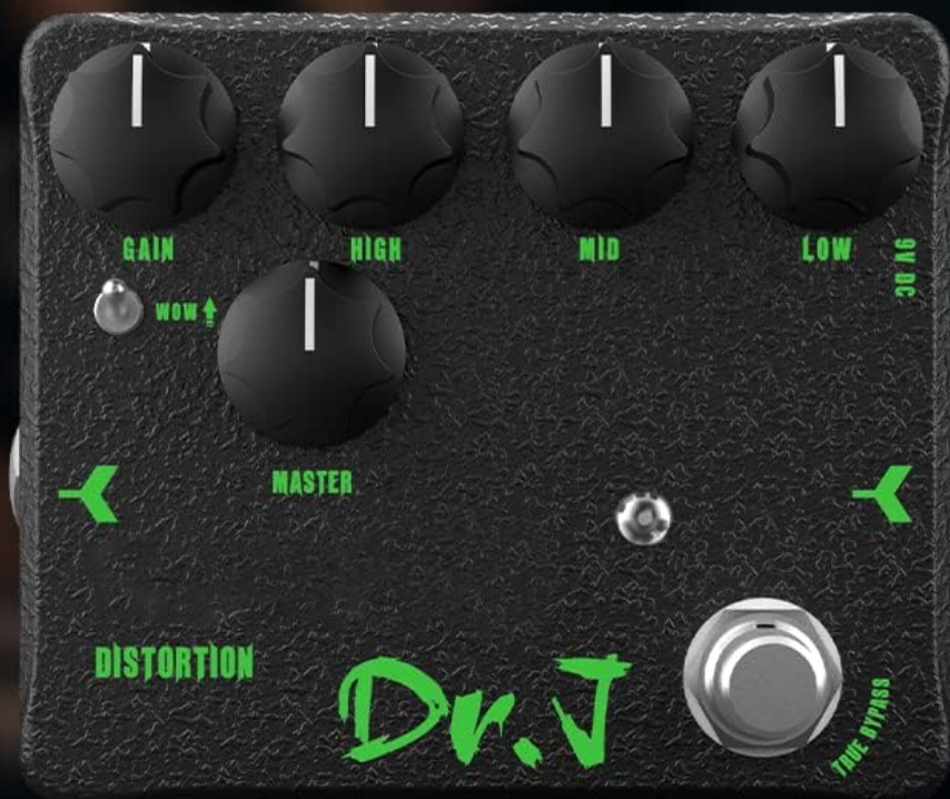
Image: Front view of the JOYO D58 Modern Metal Distortion Pedal, showing the GAIN, HIGH, MID, LOW, MASTER knobs, and the WOW CLIP switch.
