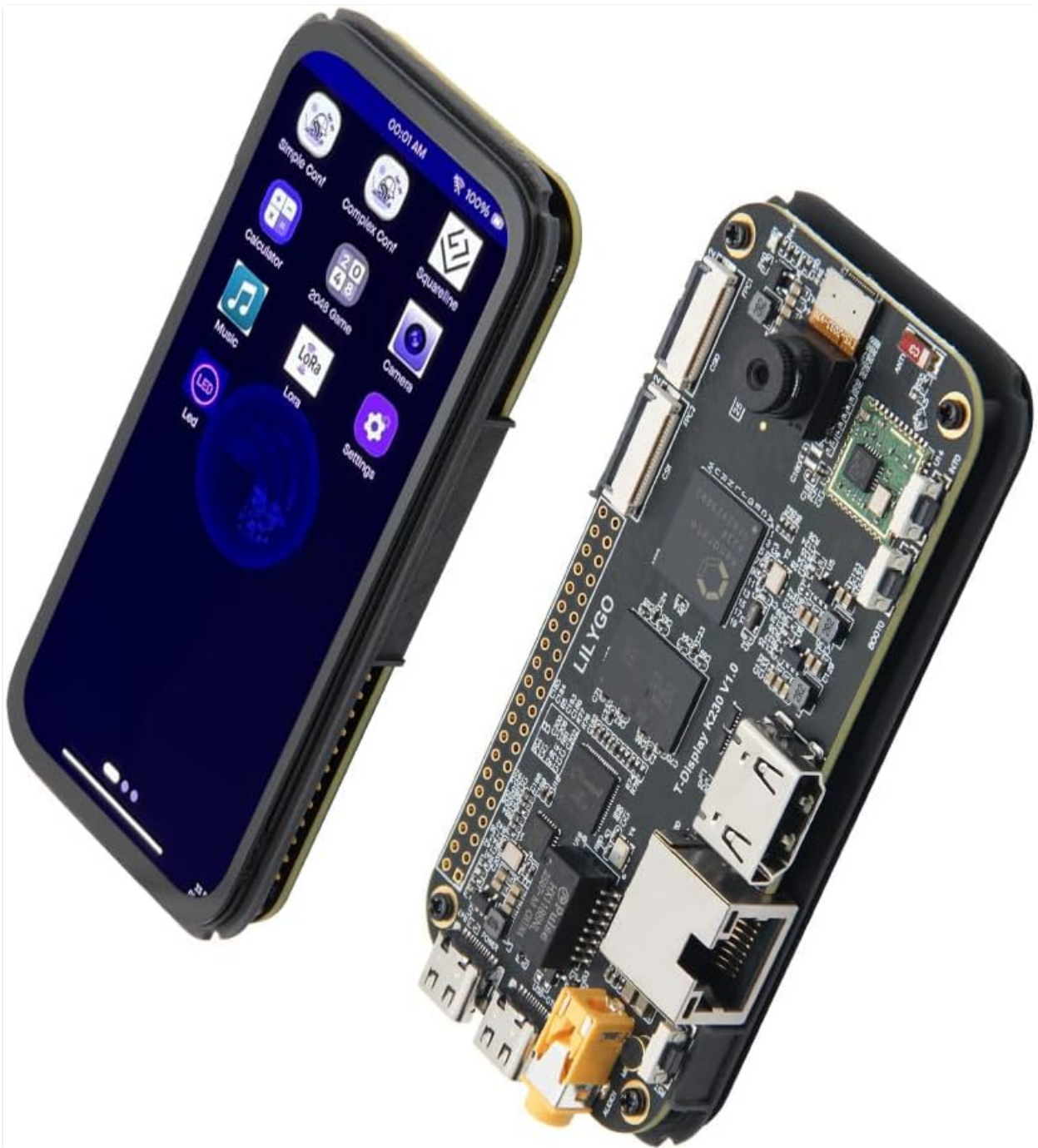
Figure 2.2: Exploded view of the T-Display K230, highlighting the main board and display assembly.
