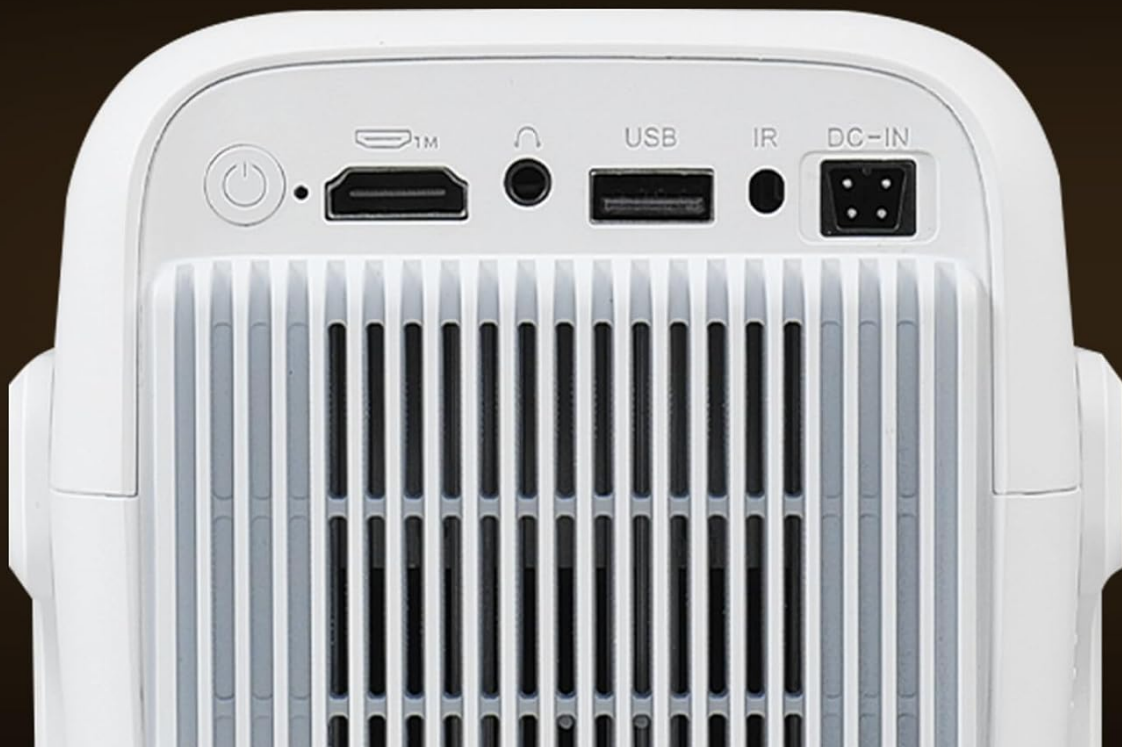
The rear panel of the LYNCAST N300 projector, displaying various input and output ports including HDMI, USB, IR receiver, and DC-IN.
