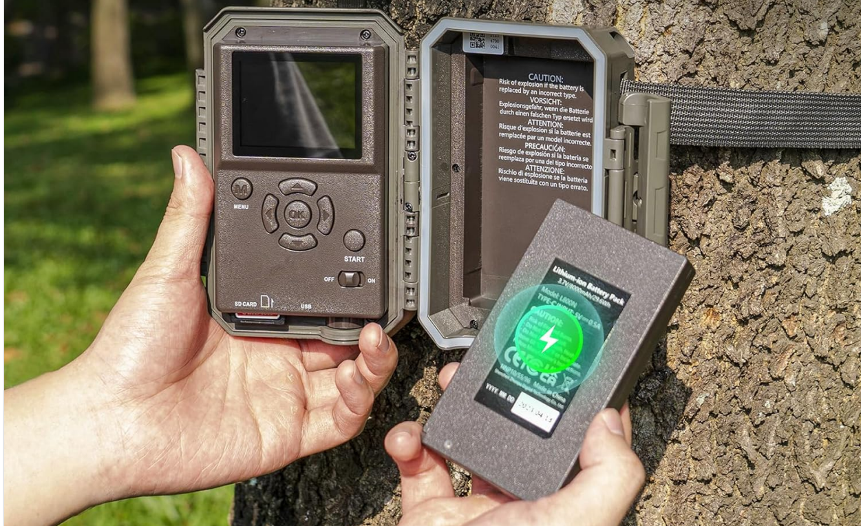
Image: A hand inserting the 8000mAh rechargeable battery pack into the open battery compartment of the GardePro X60 Pro Max camera.
