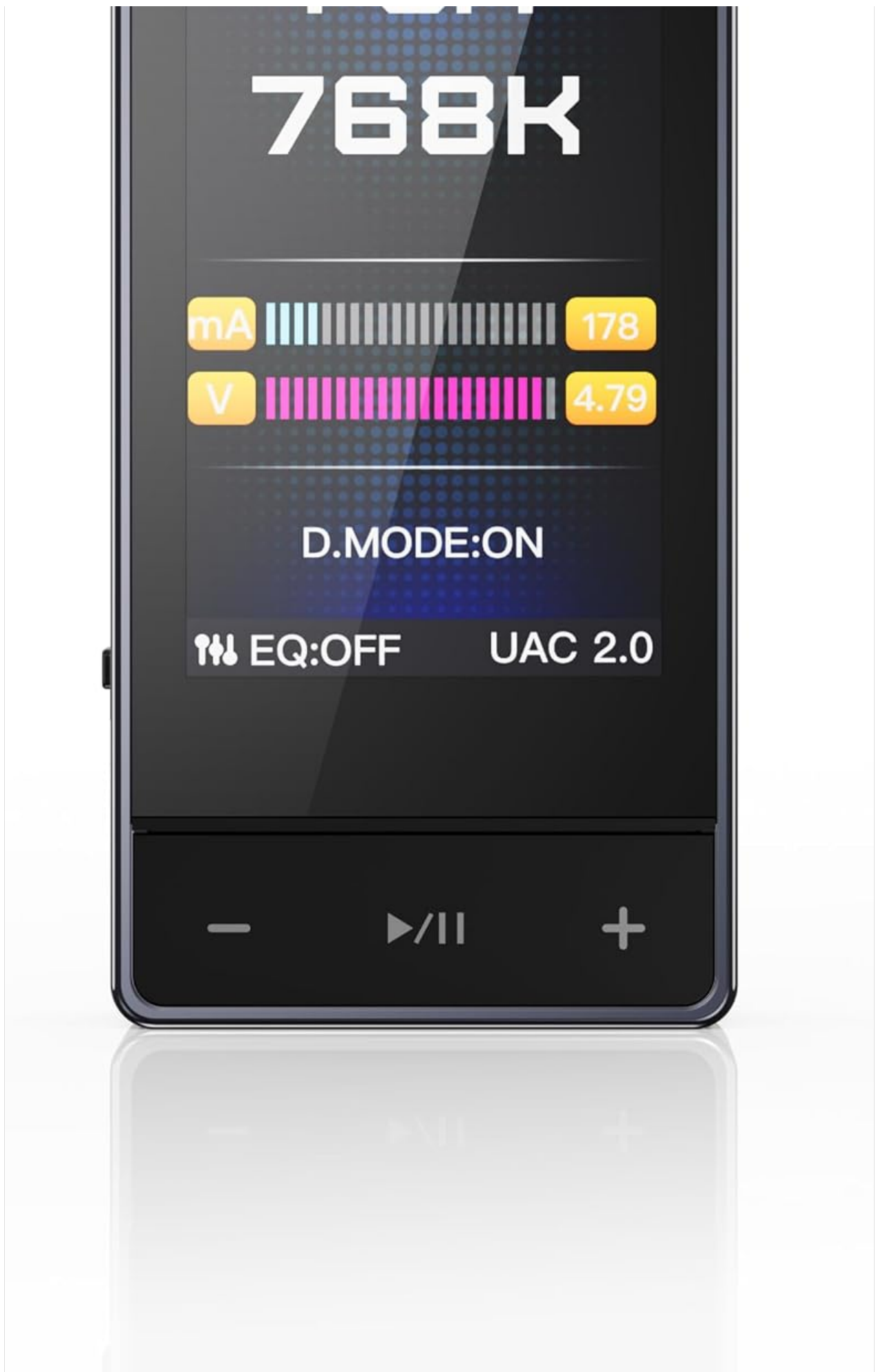
Image: Front view of the FiiO QX13, showing its vibrant color display with audio information such as PCM 768K, current, and voltage levels, along with touch controls.
