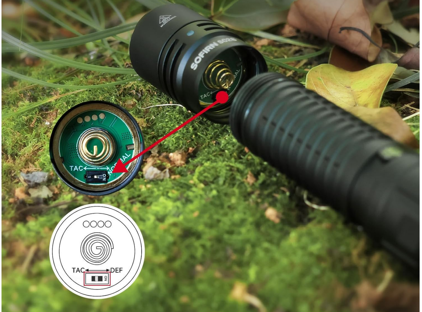
Image: A close-up view of the Sofirn SC28 flashlight with its head unscrewed, revealing the internal driver board and a micro switch labeled 'TAC' and 'DEF' for switching between user interfaces.
