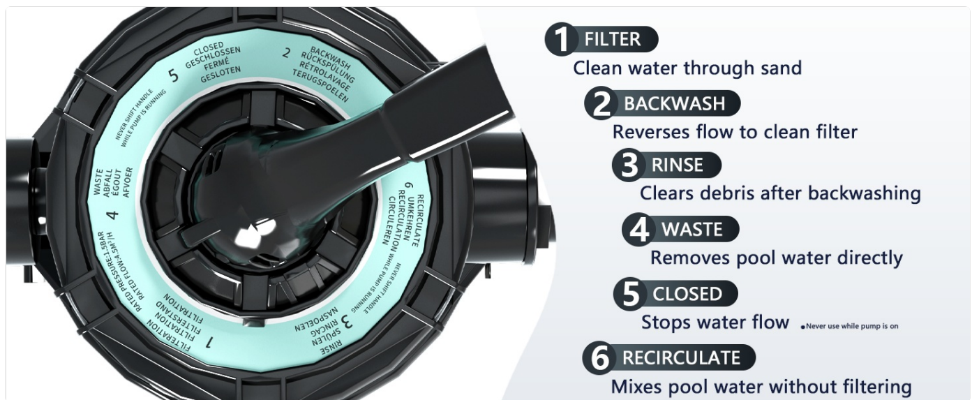
Figure 5: Multi-Port Valve Settings
