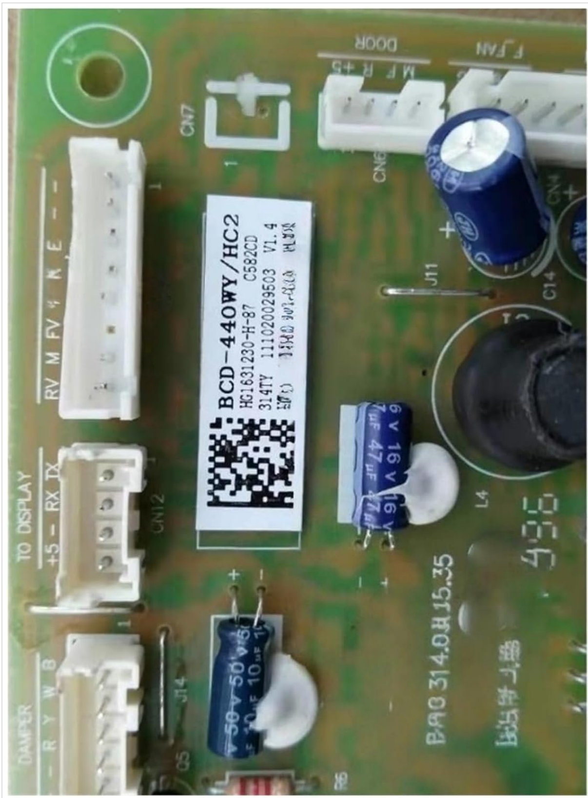
Image 1: The BCD-440WY/HC power supply board. This image shows the layout of the board with various connectors (CN7, CN6, CN12, J14) and components like capacitors and resistors. The model number "BCD-440WY/HC2" is visible on a label. This visual aid helps in identifying the correct replacement part and understanding its physical connections during installation.
