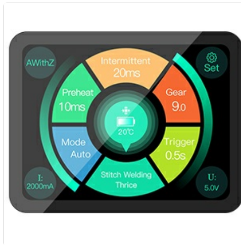
Image: A close-up of the AWithZ U3 Pro's 2-inch color LCD screen, showing the circular user interface with settings such as Intermittent (20ms), Preheat (10ms), Mode (Auto), Stitch Welding (Thrice), Gear (9.0), Trigger (0.5s), and current/voltage indicators.
