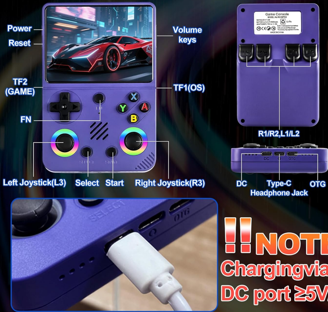
Figure 4.1: Front, back, and top views of the RG36PRO with labeled components.
