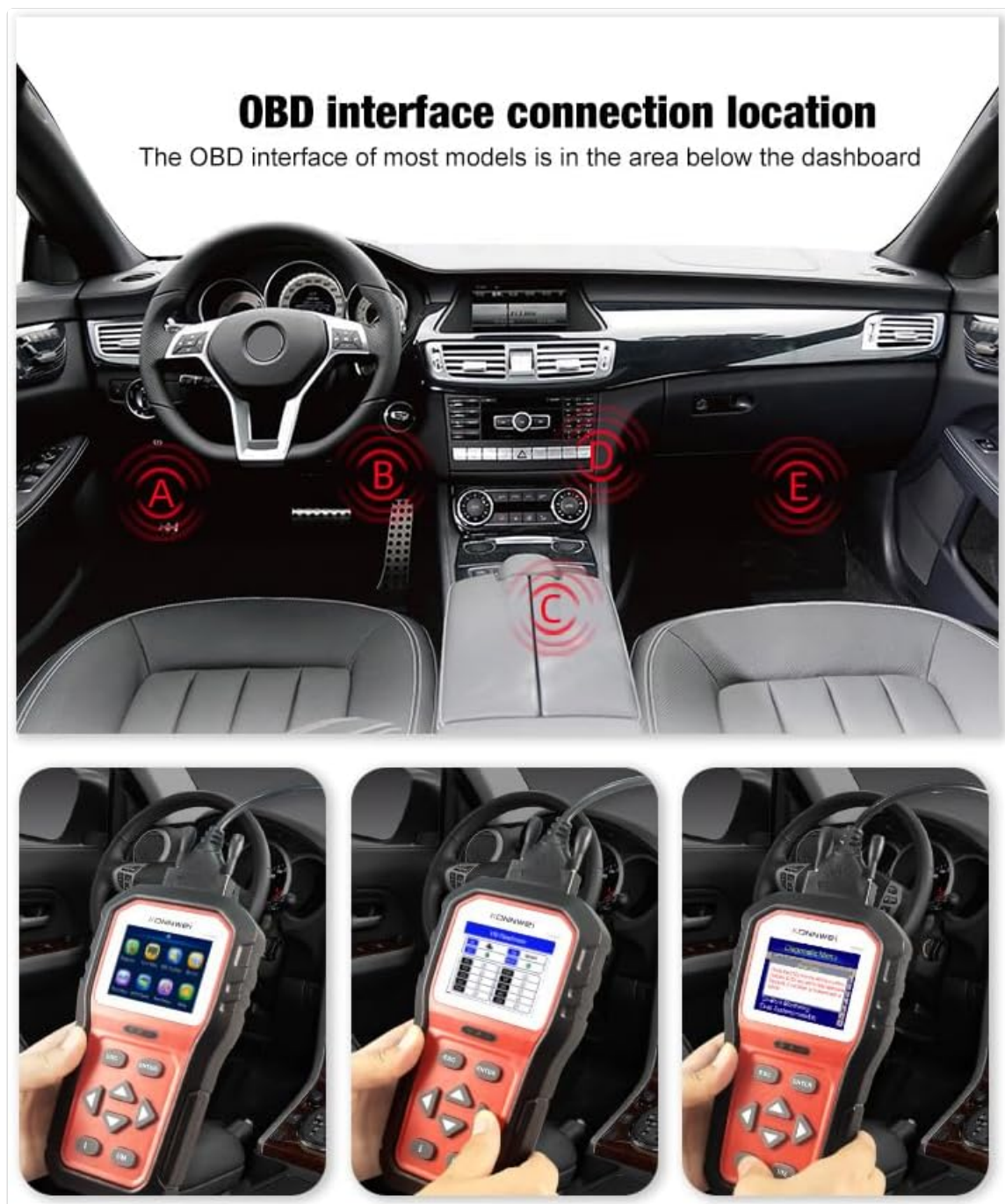
Image 3.1: Common locations for the OBDII port within a vehicle's interior, usually beneath the dashboard.
