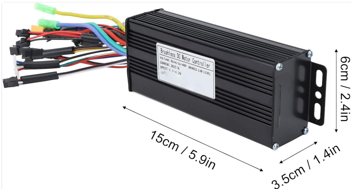
Figure 2: Controller dimensions: approximately 150mm (5.9in) length, 60mm (2.4in) width, and 35mm (1.4in) height. These dimensions help in selecting a suitable mounting location.
