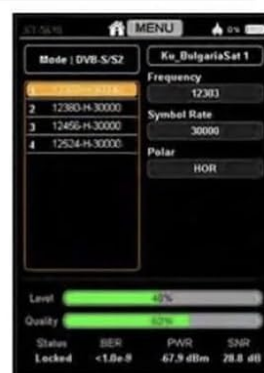
Image 2.1: A visual representation of the ST-5810's key features, including multi-standard compatibility and advanced analysis functions.
