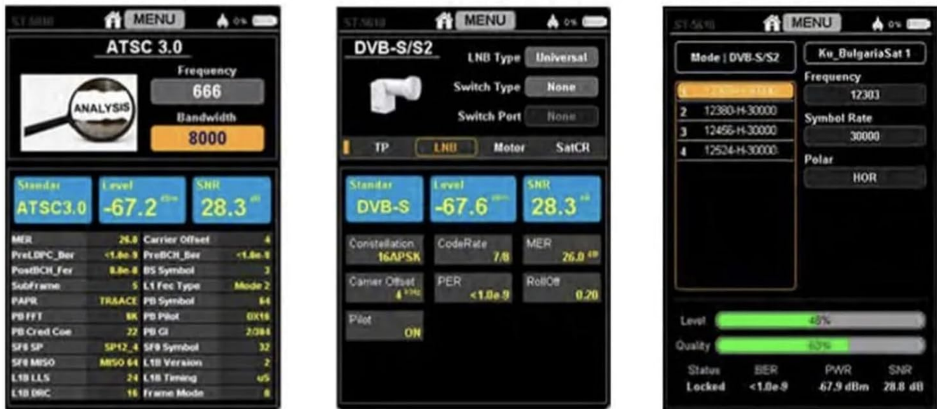
Image 5.2: Detailed measurement screens showing parameters for ATSC 3.0 and DVB-S/S2 signals, including frequency, bandwidth, SNR, and MER.
