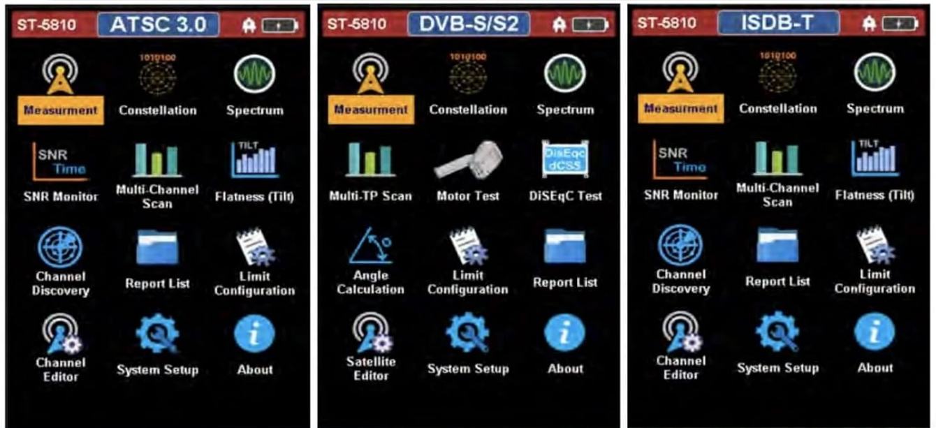
Image 5.1: Examples of the ST-5810's user interface for different TV standards, showing measurement, constellation, and spectrum options.
