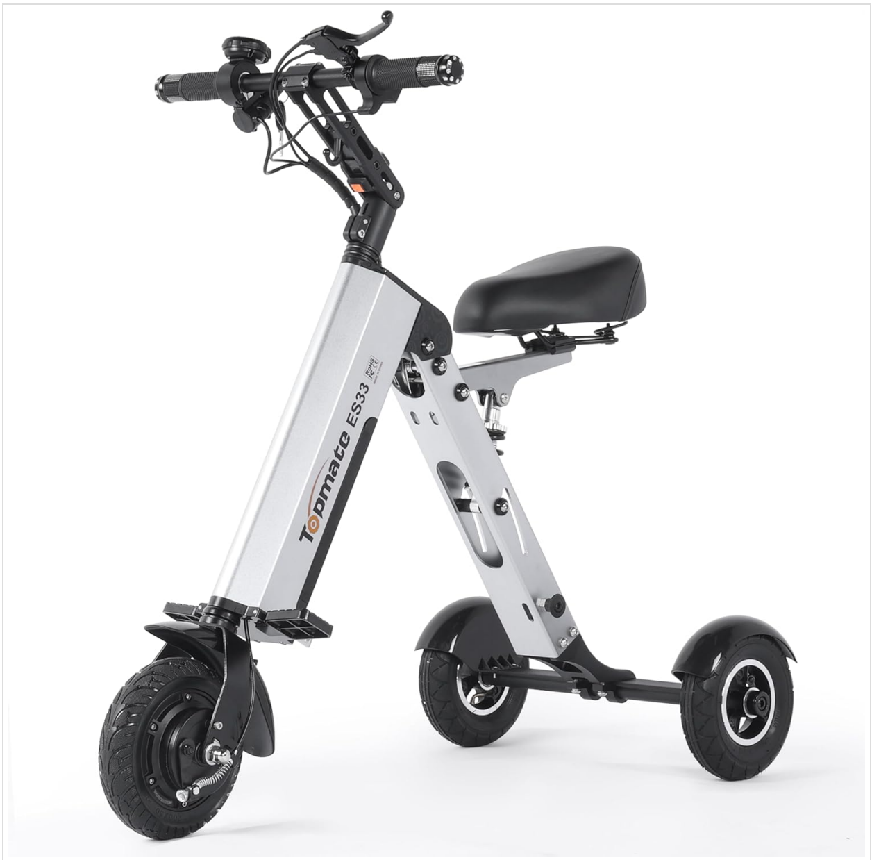
Figure 2.1: The TopMate ES33 Powered Scooter in its unfolded state, showcasing its three-wheel design, seat, and handlebars.
