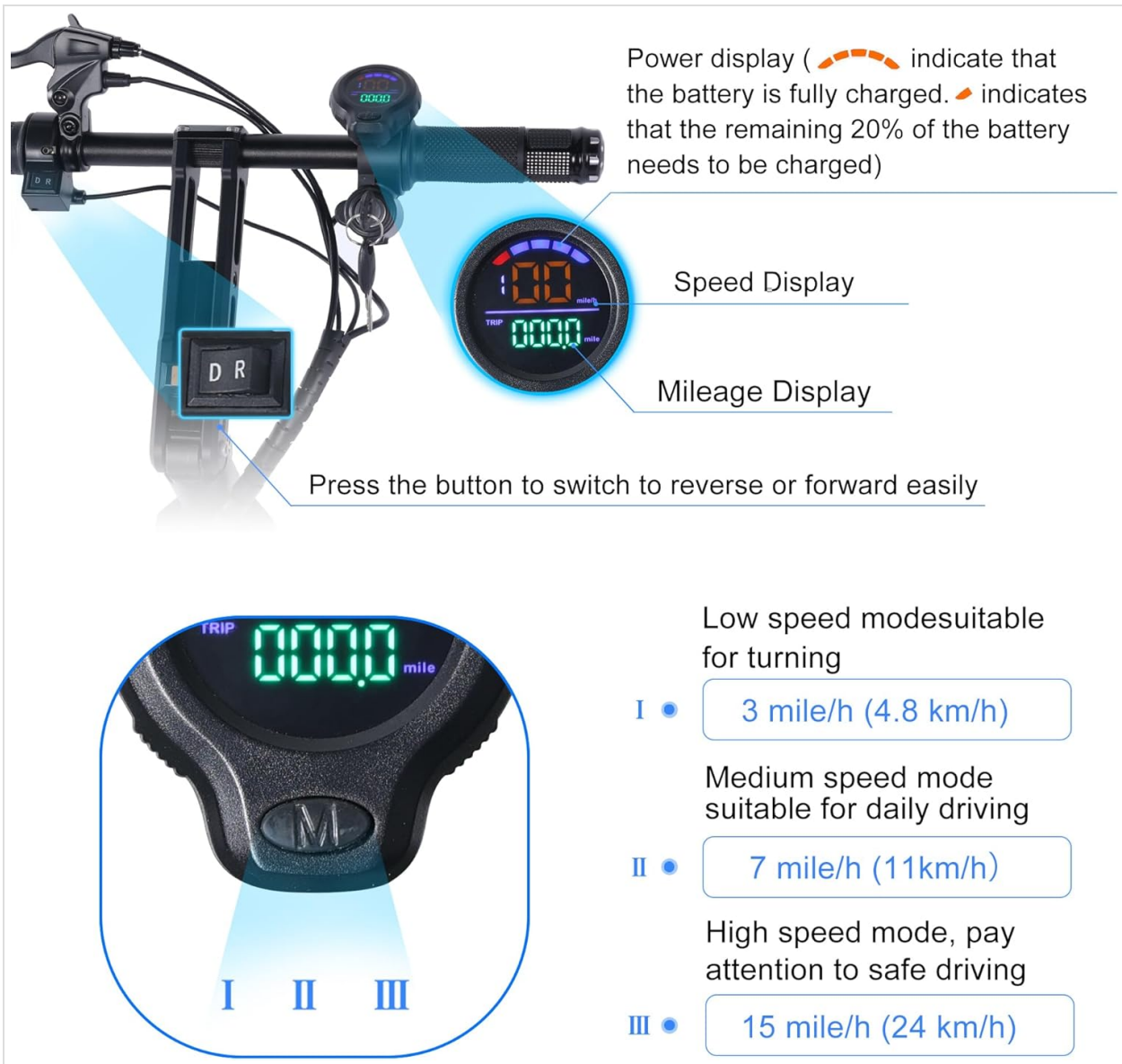
Figure 5.1: Close-up of the scooter's handlebar display, showing the power, speed, and mileage indicators, along with the D/R button for forward/reverse and the speed mode selection (I, II, III).
