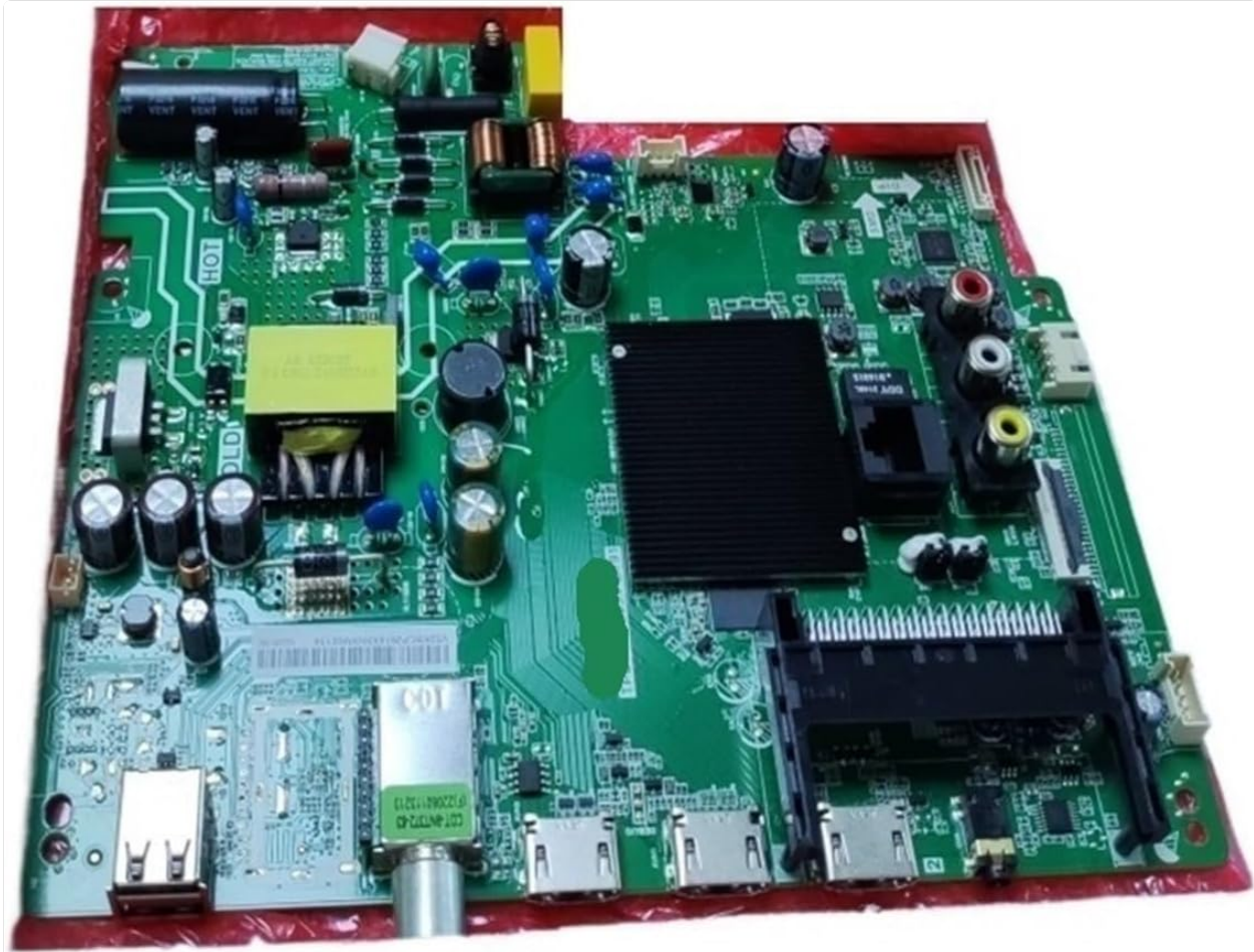
Figure 1: Top-down view of the IOAUOVEG Logic Board Inverter. This image displays the overall layout of the circuit board, highlighting the main components such as the heat sink, various capacitors, inductors, and multiple input/output ports including HDMI, USB, and network (Ethernet) connectors. The power supply section is visible on the left side.
