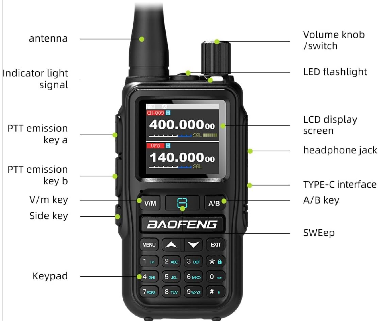
Image: Detailed diagram of the Baofeng UV-5R Mini's function keys and components.
