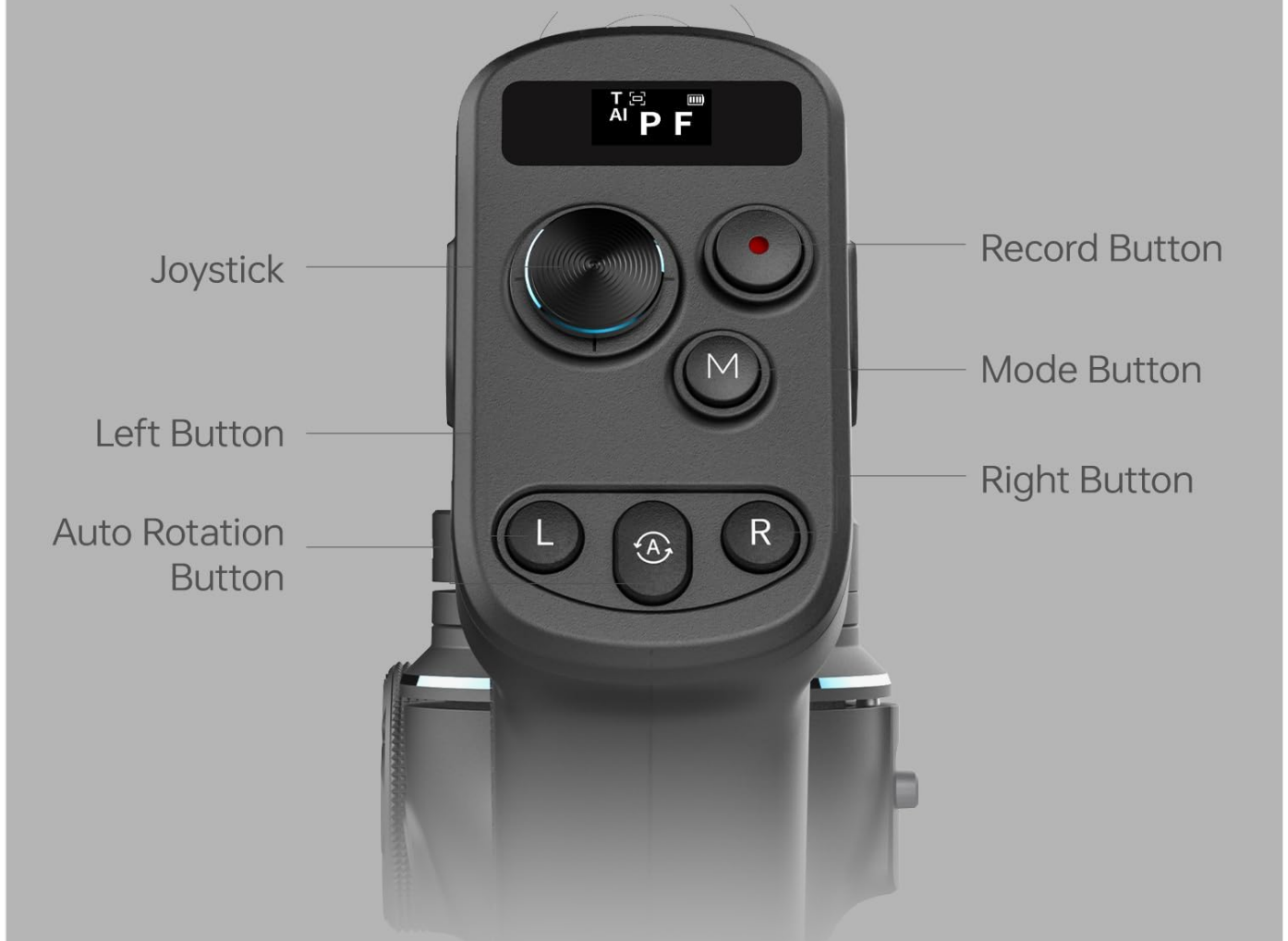
Image 4.1: Button controls and OLED status screen on the FeiyuTech SCORP-C2.
