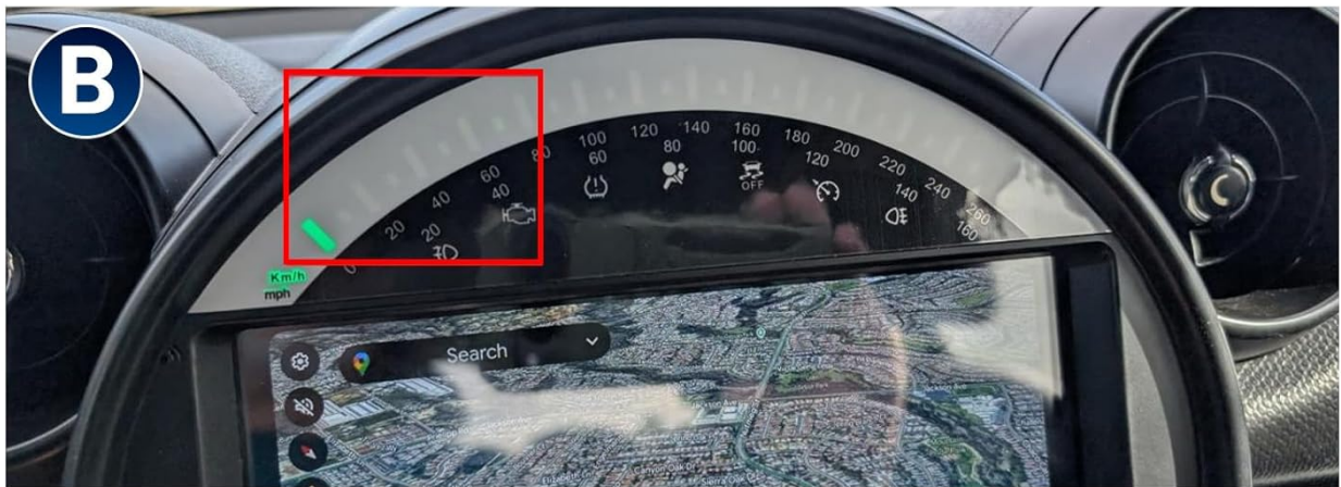
Figure: Illustration of correct (km/h) and incorrect (mph) speed unit display lighting.
