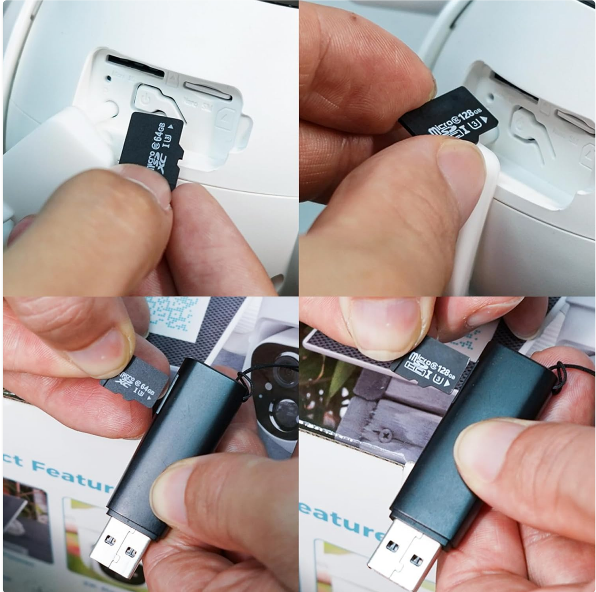
Figure 2: MicroSD Card Installation. This composite image illustrates the process of opening the camera's port, inserting a microSD card, and using a USB adapter to connect the card to a computer for data transfer.
