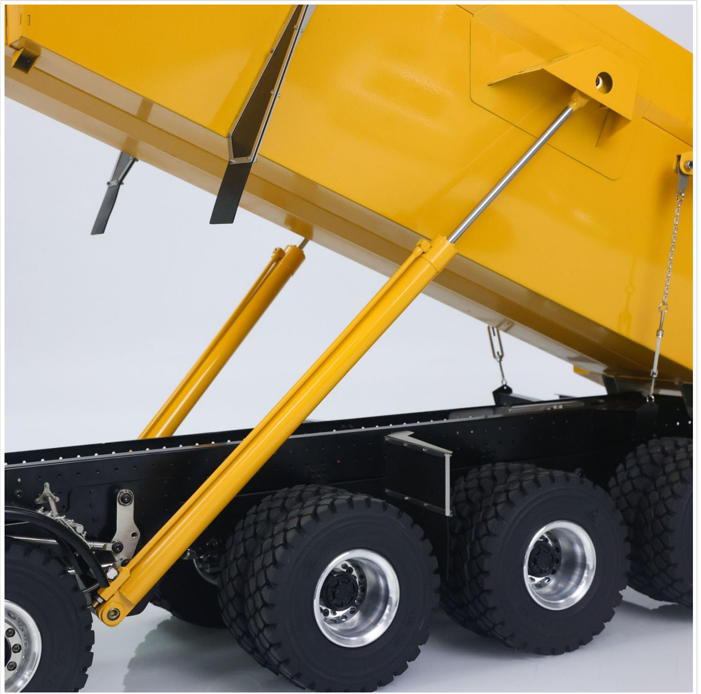
Figure 4: A close-up view of the hydraulic lift mechanism for the dumper bed. The yellow hydraulic cylinders are clearly visible, illustrating the system responsible for raising and lowering the truck's bed for material discharge.
