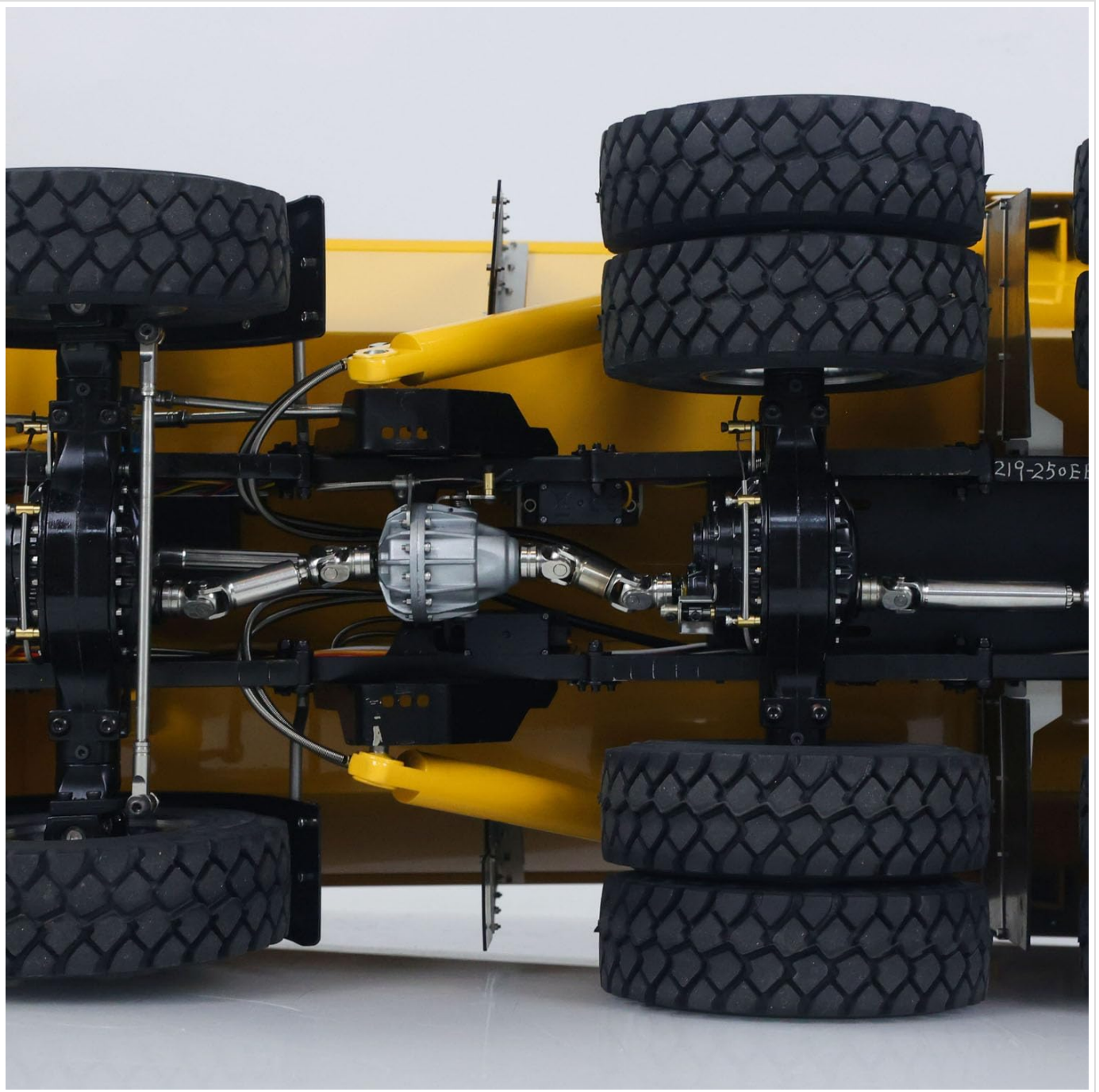
Figure 5: A detailed view of the rear axles and drivetrain components of the JDM 219 Dumper Truck. This image shows the robust metal construction of the axles and the differential lock mechanisms, crucial for its 10x10 all-wheel drive capability.
