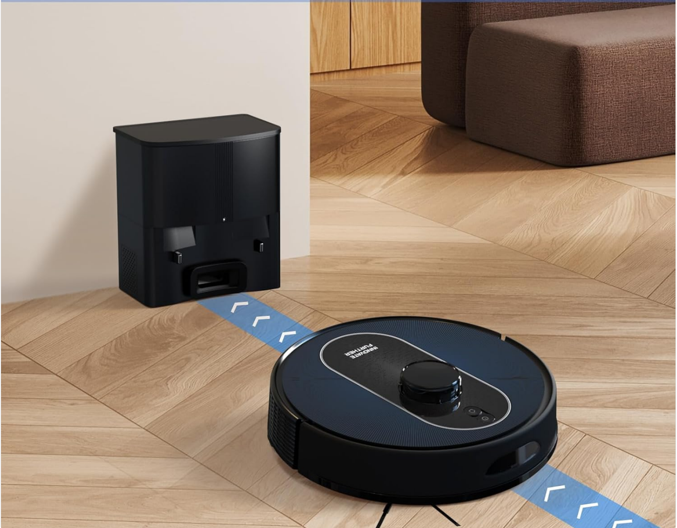
Image 5.7: The robot automatically navigates back to its charging station when its battery is low.
