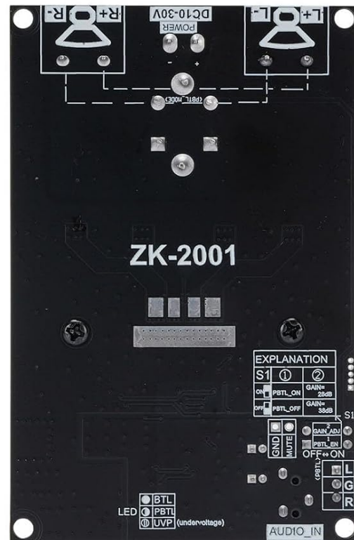
Figure 6.1: Various views of the amplifier module, including the multi-tooth heat sink and the ZK-2001 model label. This image also shows the back of the board with a window for heat dissipation.
