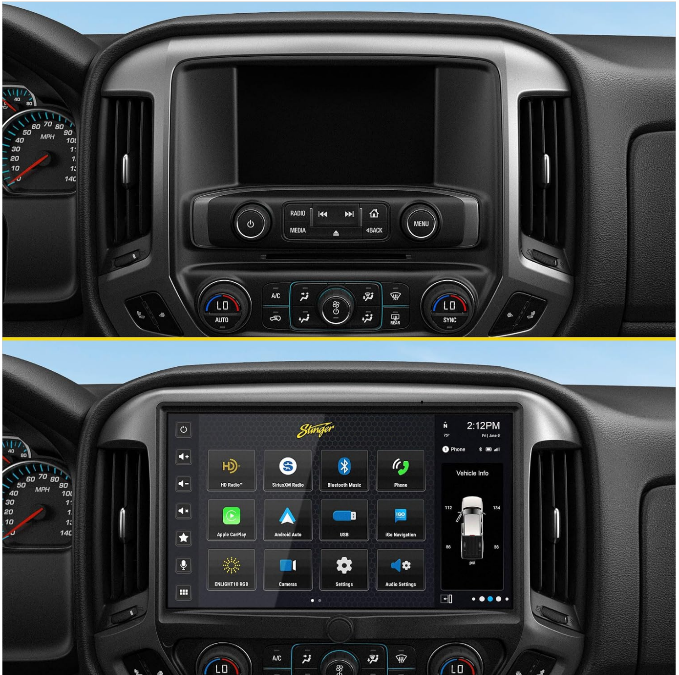
Image: Comparison of the original dashboard radio and the Stinger HORIZON12 installed, showing the integrated 12.8-inch display.
