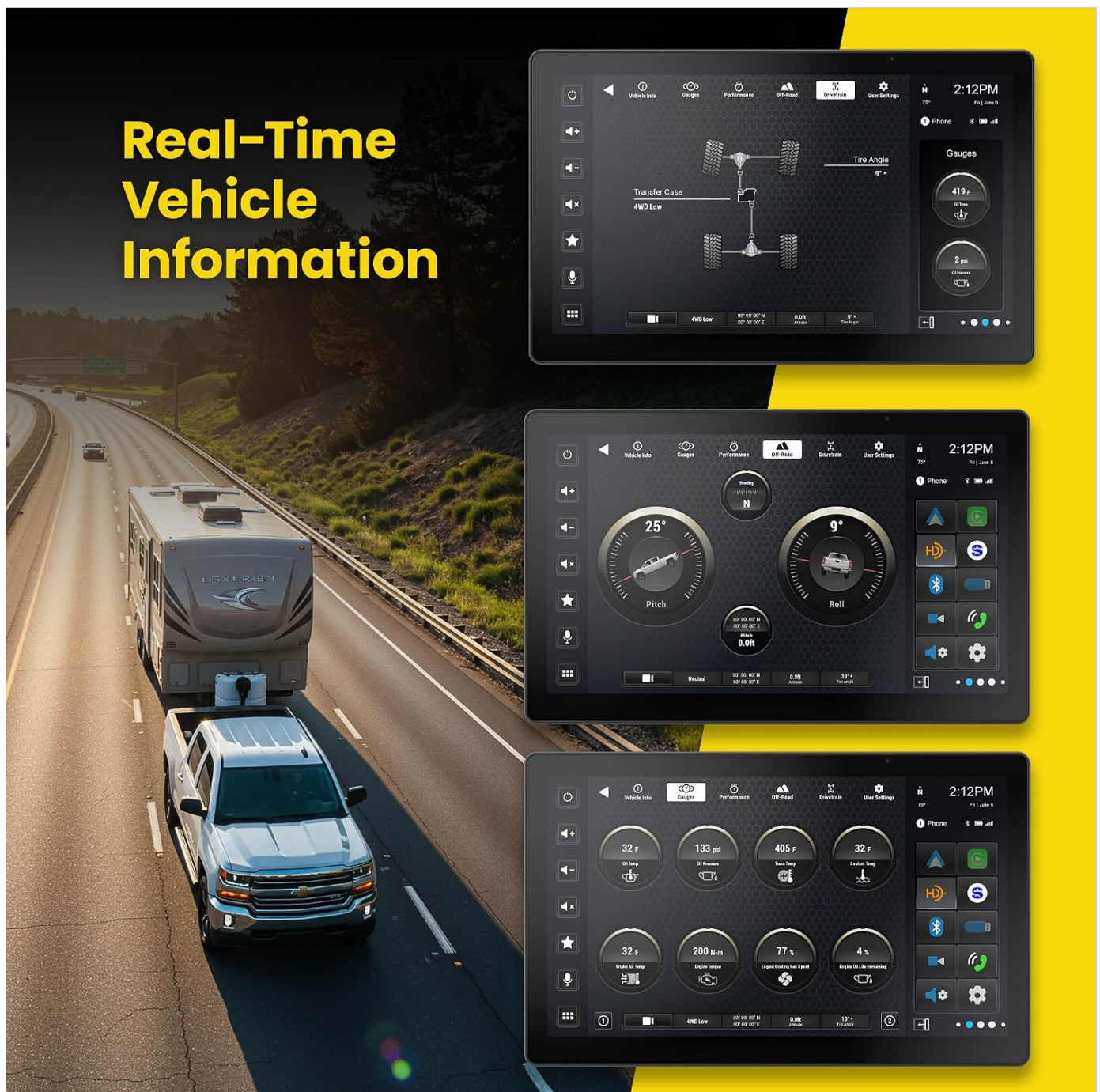
Image: The Stinger HORIZON12 screen displaying real-time vehicle information, including pitch and roll angles, and various performance gauges like oil temp and oil pressure.
