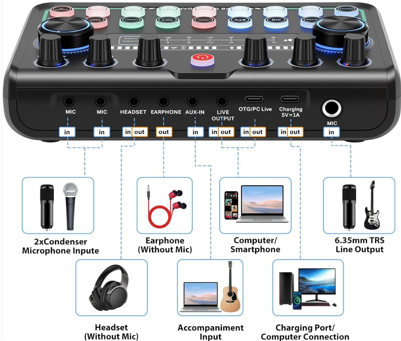
Image 2.1: All included components of the condenser microphone kit with the sound card.
