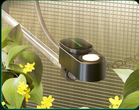
Figure 3.3: Example of a PPFD sensor connected to the system.
