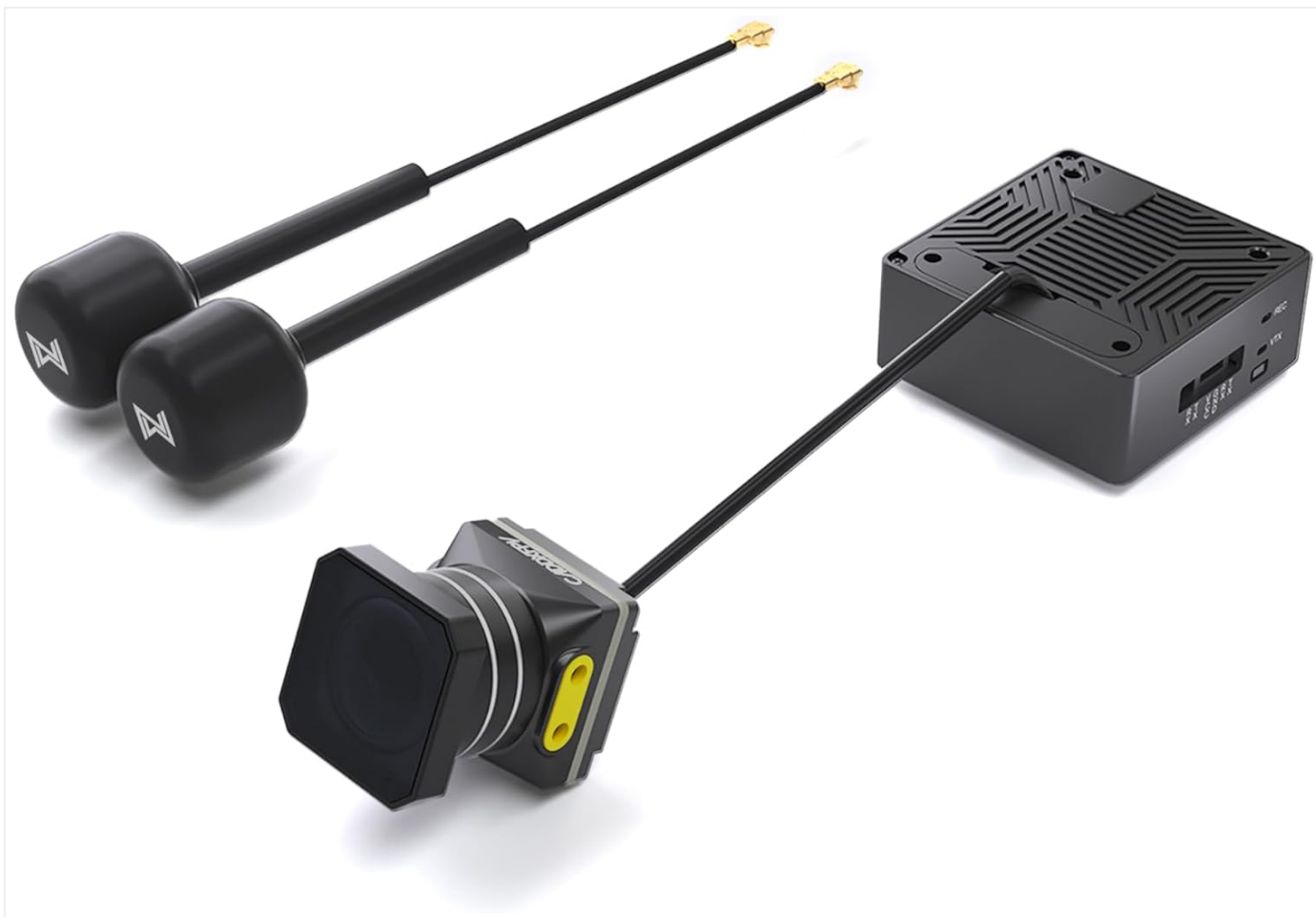
Figure 3: The Moonlight Kit, showing the camera, video transmitter (VTX) module, and two antennas.
