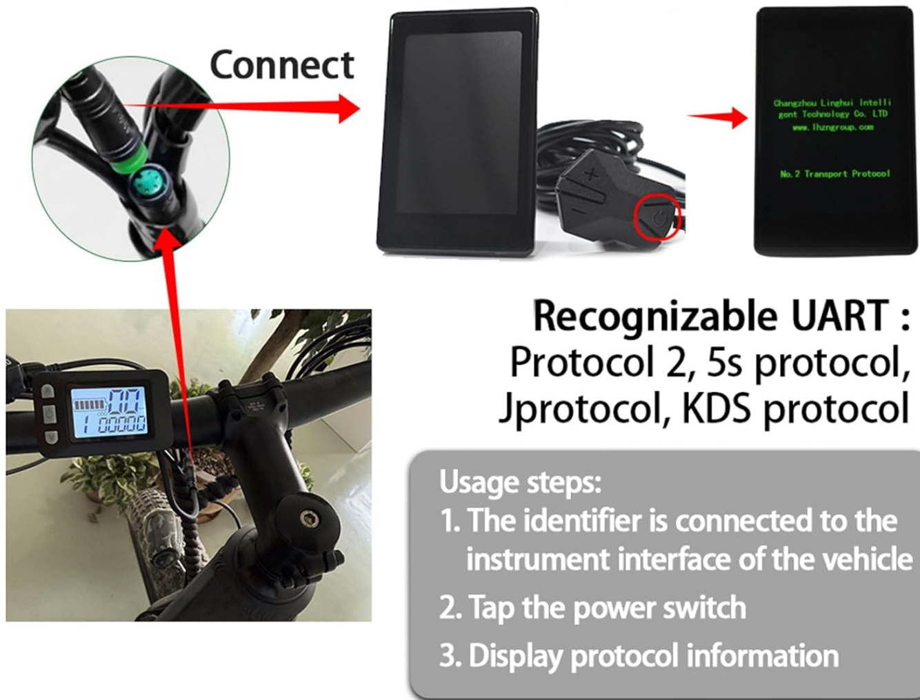
Image: Diagram illustrating the connection of the recognizer to an e-bike display for protocol identification, showing the steps and supported UART protocols.
