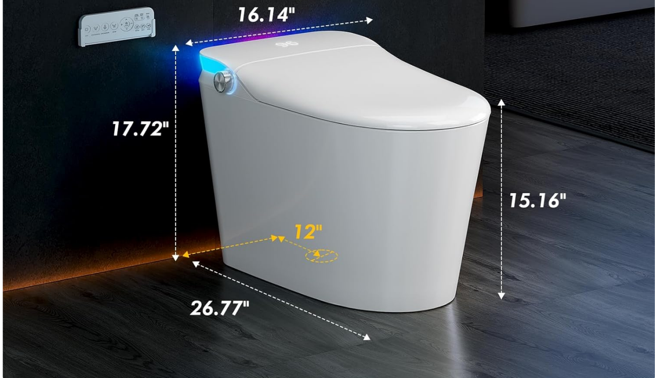
Image 5.1: Product Dimensions. This diagram provides critical measurements for installation, including depth, width, and height, and the 12-inch rough-in dimension.
