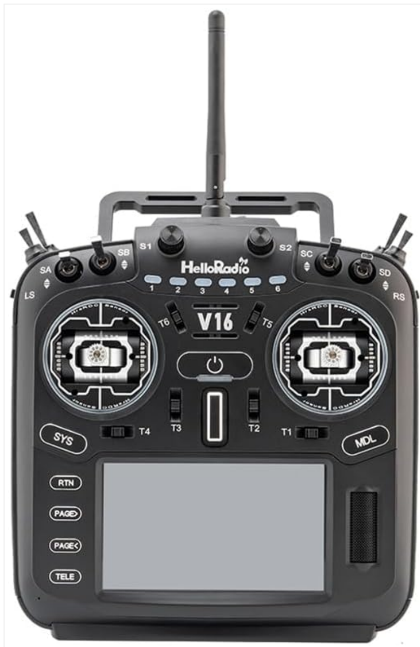
Figure 2.1: Front view of the V16 MAX ELRS Multi Protocol Transmitter. This image displays the overall layout of the transmitter, including the central power button, gimbals, switches, and the touch screen display at the bottom.
