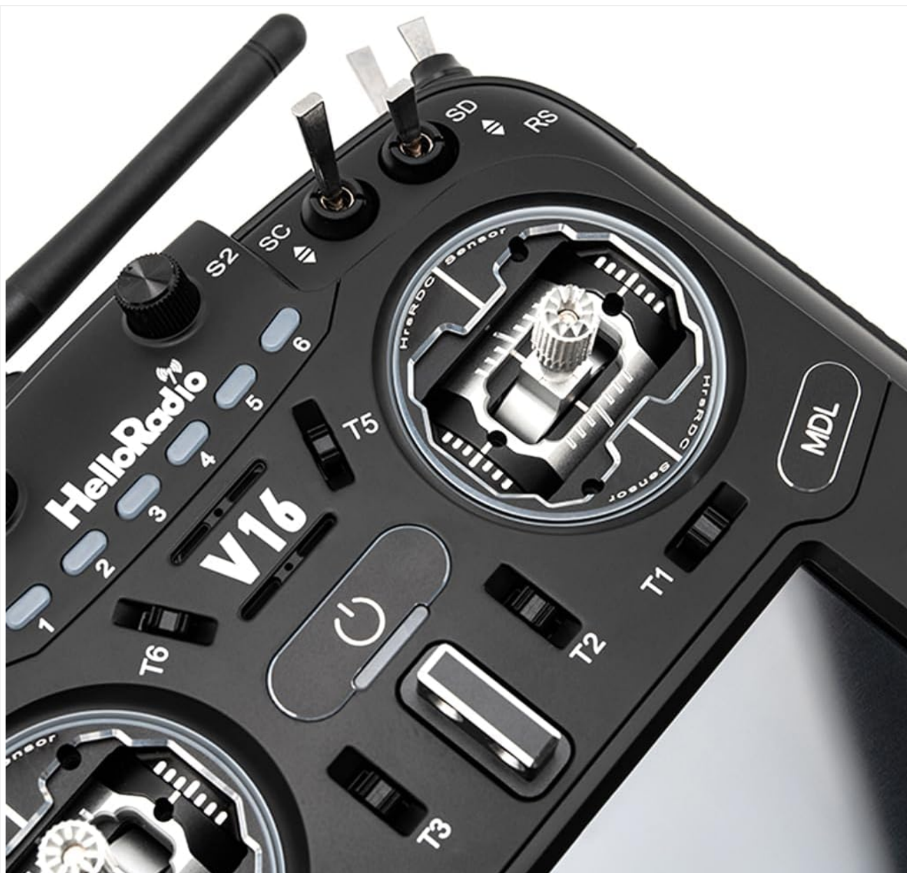
Figure 2.2: Close-up view of the right gimbal and surrounding switches (T1, T2, T5, T6) on the V16 MAX ELRS Transmitter. This highlights the precision RDC90 joystick sensor and the arrangement of control toggles.
