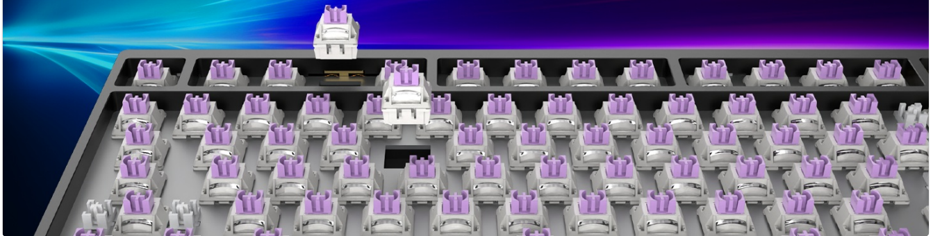
Image 4.5: A detailed view of the magnetic switches, demonstrating the 'Mix' function for easy replacement and customization.
