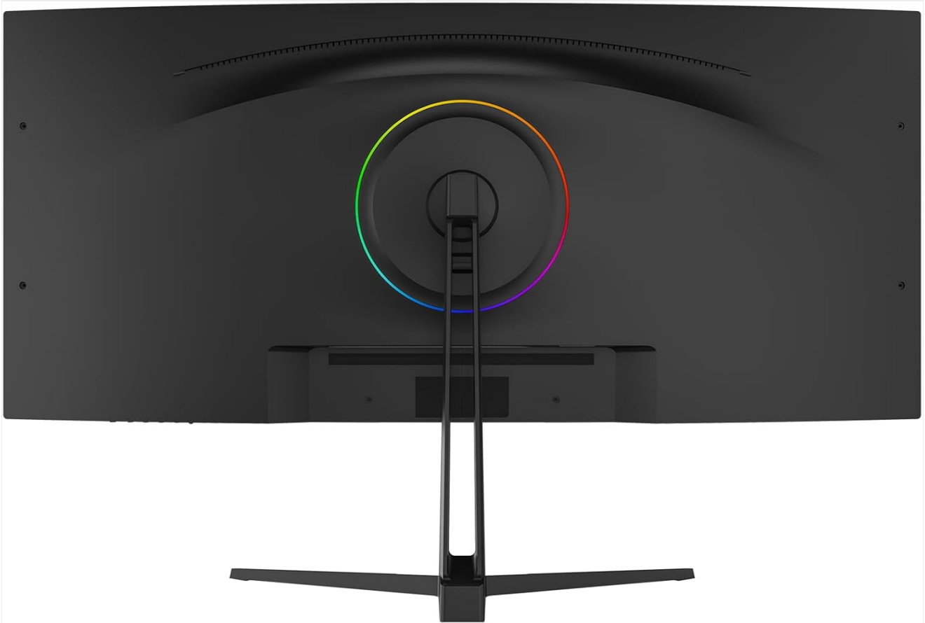
Image: Rear view of the monitor, highlighting the VESA mount compatibility and the RGB lighting ring.
