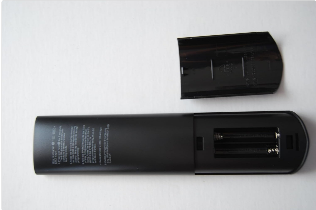
Image: Back view of the vSeeBox remote control with the battery compartment open, showing the slots for two AAA batteries.
