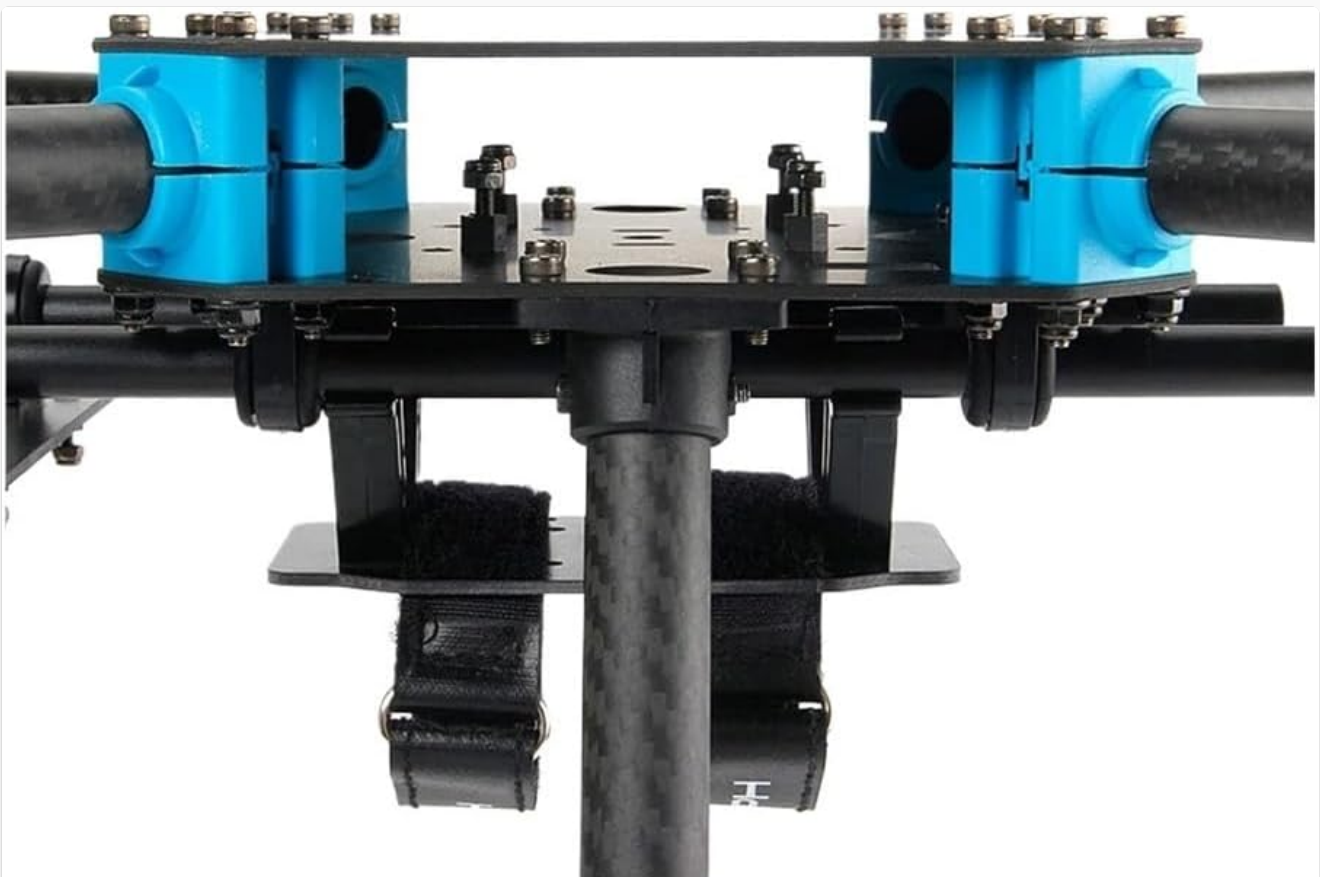
Image 4.2: Side profile showing the landing gear and the battery bracket with straps.
