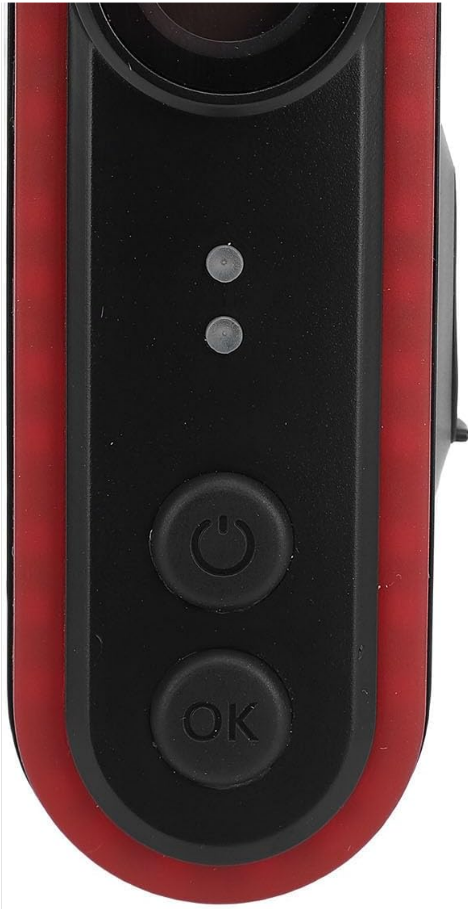
Figure 2.2: Top view of the camera, highlighting the power and OK buttons.
