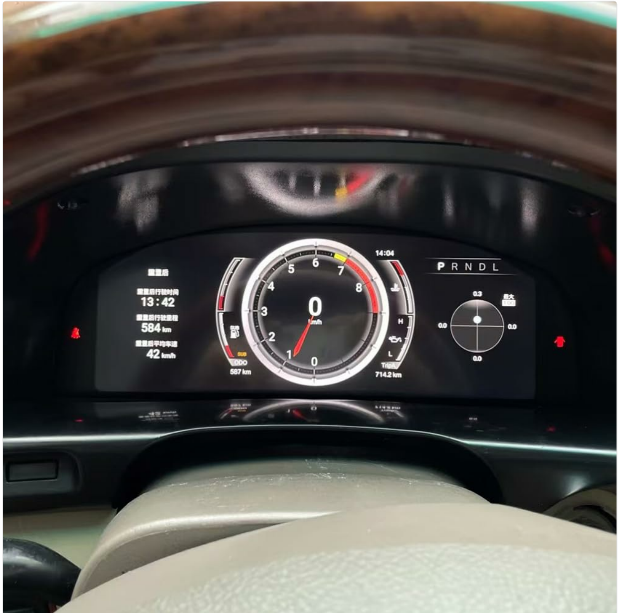
Image 3.1: The MOOKAKA 12.3-inch Digital Instrument Cluster actively displaying various vehicle parameters such as speed, engine RPM, current gear, time, and other essential driving information within a vehicle's dashboard.
